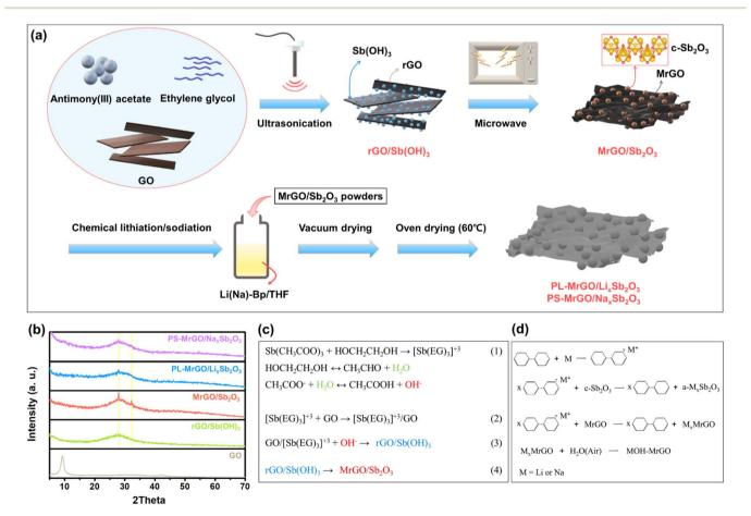
Fig. 1 (a) Schematic representation of the synthesis route for PL(S)-MrGO/Li(Na)<sub>x</sub>Sb<sub>2</sub>O<sub>3</sub> composites. (b) X-ray diffraction (XRD) patterns of GO, MrGO/Sb(OH)<sub>3</sub>, MrGO/Sb<sub>2</sub>O<sub>3</sub>, PL-MrGO/Li<sub>x</sub>Sb<sub>2</sub>O<sub>3</sub>, and PS-MrGO/Na<sub>x</sub>Sb<sub>2</sub>O<sub>3</sub>. (c) Chemical reactions during the synthesis of MrGO/Sb<sub>2</sub>O<sub>3</sub>. (d) Chemical reactions during the pre-lithiation/sodiation process.
