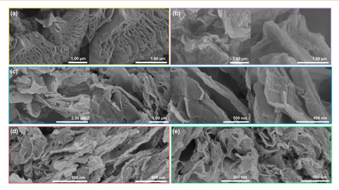
Fig. 2 (a) Field emission scanning electron microscopy (FE-SEM) images of (a) MrGO, (b) EG-MGO, (c) MrGO/Sb<sub>2</sub>O<sub>3</sub>, (d) PL-MrGO/Li<sub>x</sub>Sb<sub>2</sub>O<sub>3</sub>, and (e) PS-MrGO/Na<sub>x</sub>Sb<sub>2</sub>O<sub>3</sub>
