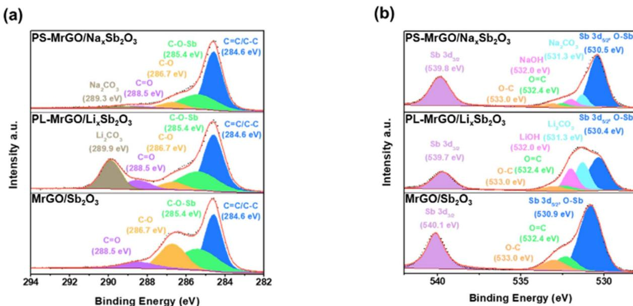
Fig. 3 High-resolution XPS spectra of (a) C 1s and (b) Sb 3d & O 1s for  $\text{MrGO}/\text{Sb}_2\text{O}_3$ , PL-MrGO/ $\text{Li}_x\text{Sb}_2\text{O}_3$ , and PS-MrGO/ $\text{Na}_x\text{Sb}_2\text{O}_3$ .
