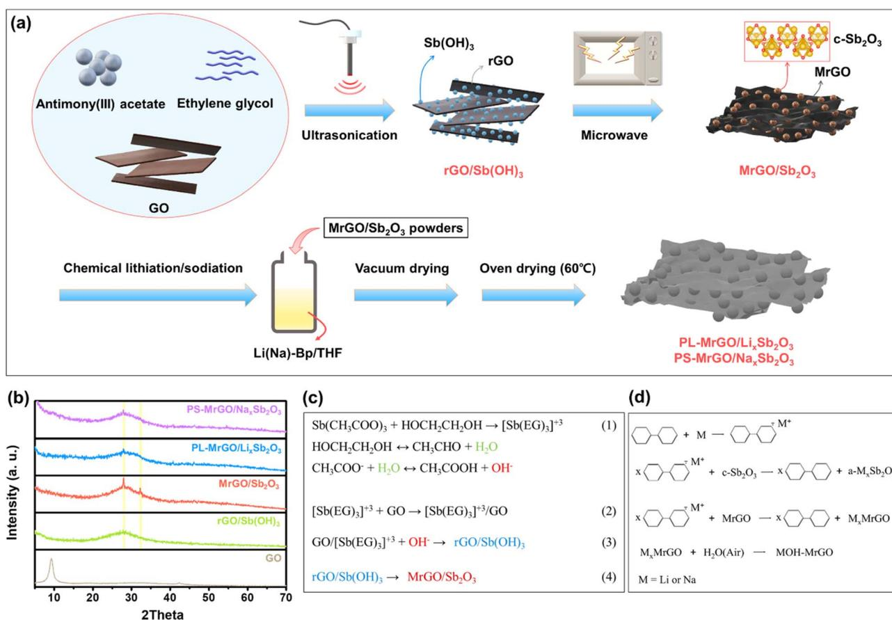
Fig. 1 (a) Schematic representation of the synthesis route for PL(S)-MrGO/Li(Na)<sub>x</sub>Sb<sub>2</sub>O<sub>3</sub> composites. (b) X-ray diffraction (XRD) patterns of GO, MrGO/Sb(OH)<sub>3</sub>, MrGO/Sb<sub>2</sub>O<sub>3</sub>, PL-MrGO/Li<sub>x</sub>Sb<sub>2</sub>O<sub>3</sub>, and PS-MrGO/Na<sub>x</sub>Sb<sub>2</sub>O<sub>3</sub>. (c) Chemical reactions during the synthesis of MrGO/Sb<sub>2</sub>O<sub>3</sub>. (d) Chemical reactions during the pre-lithiation/sodiation process.
