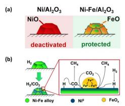
Fig. 10 (a) Deactivation of a monometallic Ni-based catalyst and the protective role of "sacrificial" iron in a NiFe catalyst during dynamic methanation of CO<sub>2</sub> (this figure has been reproduced from ref. 81 with permission from Wiley, copyright 2019). (b) Scheme representation of the CO<sub>2</sub> activation mechanism on Ni-Fe alloy-based catalysts during methanation reaction (this figure has been reproduced from ref. 93 with permission from RSC, copyright 2020).
