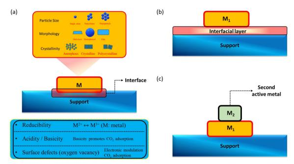
Fig. 7 The schematic representation of factors affecting the catalytic performance of heterogeneous catalysts in  $CO_2$  methanation. Here "M" stands for the active metal. (a) The parameters of active metal affecting the catalytic performance, (b) the interfacial layer and (c) the additive of second metal.
