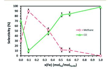
Fig. 11 Effect of Fe content on CH<sub>4</sub> and CO selectivity in comparison to sole metals (this figure has been reproduced from ref. 82 with permission from RSC, copyright 2018).
