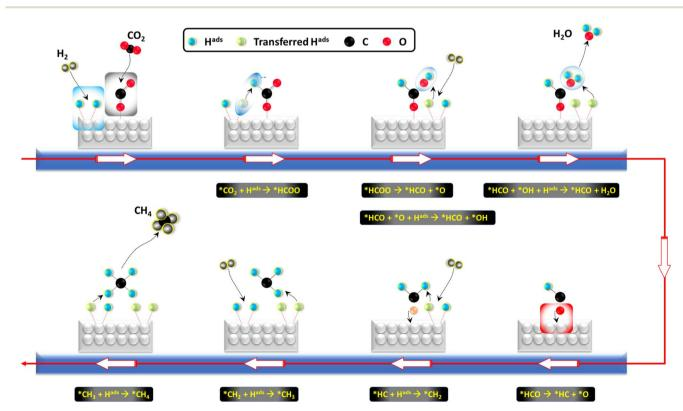
Fig. 4 The formate reaction pathway of CO<sub>2</sub> methanation.
