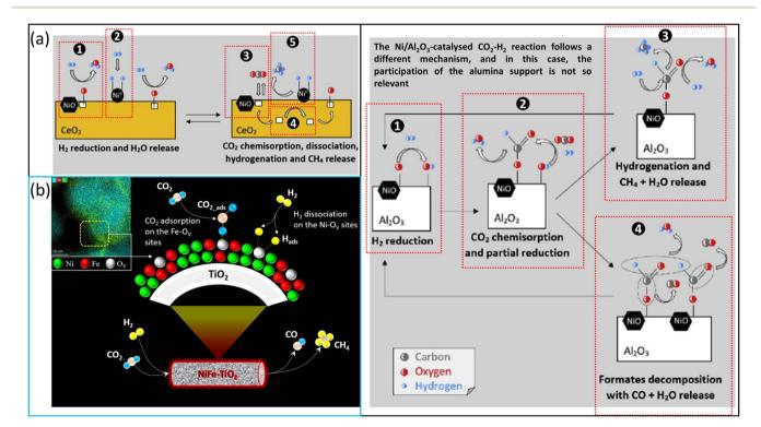
Fig. 14 The CO<sub>2</sub> methanation reaction pathways on (a) CeO<sub>2</sub> and  $Al_2O_3$  support (this figure has been reproduced from ref. 112 with permission from Elsevier, copyright 2020). (b) The schematic representation of NiFe-TiO2 catalyst (this figure has been reproduced from ref. 14 with permission from Elsevier, copyright 2024).
