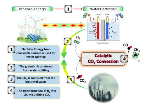
Fig. 1 Schematic representations of the closed carbon loop.
