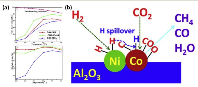
Fig. 13 (a) The  $CO_2$  conversion and  $CH_4$  selectivity versus reaction temperature over OMA-10Ni, OMA-2Co8Ni, and OMA-10Co catalysts. (b) The proposed synergistic mechanism between Co and Ni domains over the OMA-xCoyNi catalysts toward CO2 methanation (this figure has been reproduced from ref. 84 with permission from Elsevier, copyright 2018).
