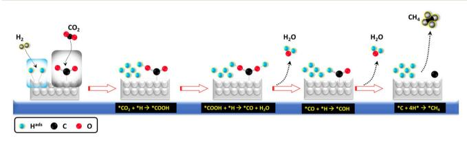
Fig. 5 The carboxyl pathway of CO<sub>2</sub> methanation.
