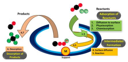
Fig. 2 The reaction pathways for heterogeneous catalytic CO<sub>2</sub> methanation.
