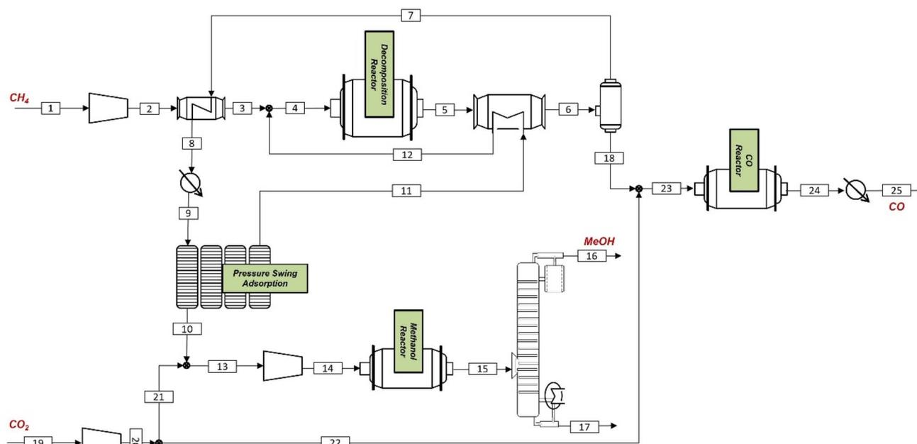
Fig. 1 Schematic of the MeOH and CO co-production plant.
