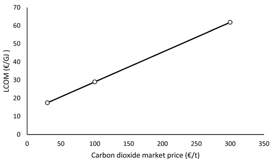
Fig. 3 Carbon dioxide market price on the levelised cost of methanol production.
