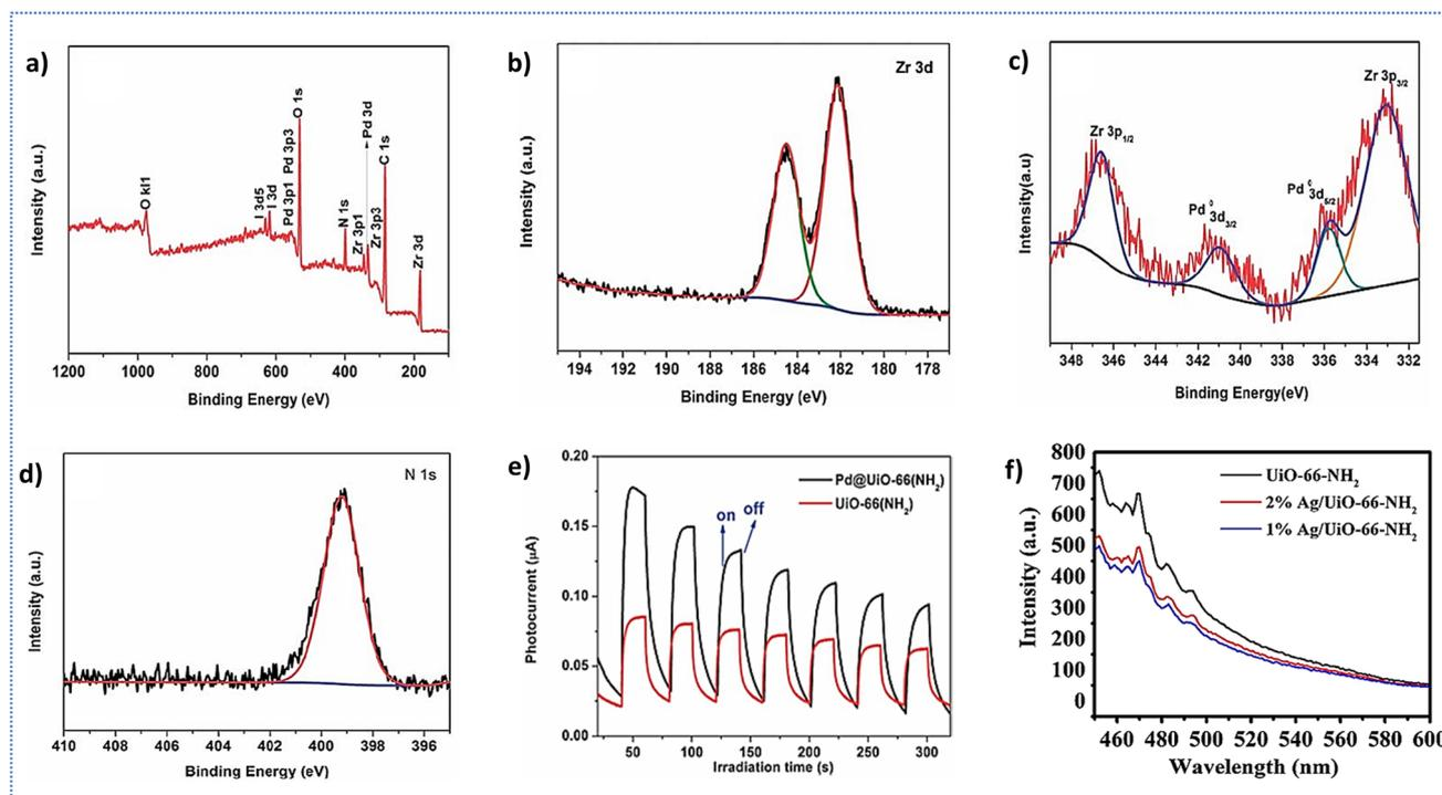
Fig. 9 (a)–(d) XPS spectra of Pd@UiO-66(NH<sub>2</sub>). (e) transient photocurrent response of UiO-66(NH<sub>2</sub>) and Pd@UiO-66(NH<sub>2</sub>), reproduced with permission from The Royal Society of Chemistry. Copyright © 2013.<sup>49</sup> and (f) PL spectra of UiO-66-NH<sub>2</sub>, 1% Ag/UiO-66-NH<sub>2</sub>, and 2% Ag/UiO-66-NH<sub>2</sub>, reproduced with permission from Springer. Copyright © 2019.<sup>96</sup>
