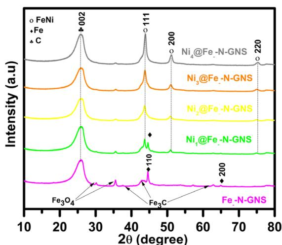
Fig. 1 XRD patterns of  $\text{Ni}_1\text{@Fe-N-GNS}$ ,  $\text{Ni}_2\text{@Fe-N-GNS}$ ,  $\text{Ni}_3\text{@Fe-N-GNS}$ ,  $\text{Ni}_4\text{@Fe-N-GNS}$ , and Fe-N-GNS (synthesized without the nickel precursor).
