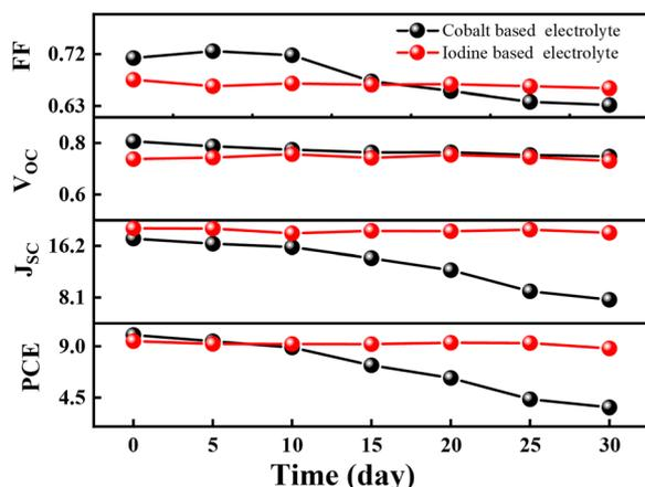
Fig. 6 Stability trial TZ1-based DSSCs using cobalt and iodine-based electrolytes at 60 °C.
