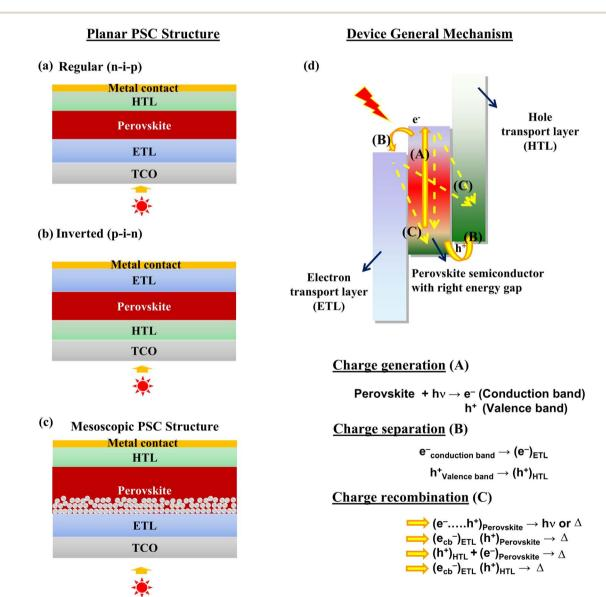
Fig. 1 The schematic illustration details the sandwich structure of a perovskite solar cell in two configurations: n-i-p and p-i-n (a and b). It further illustrates the n-i-p configuration with a mesoporous structure (c), and demonstrates the process of charge generation under light, highlighting potential charge recombination pathways, including radiative  $(h\nu)$  and thermal  $(\Delta)$  recombinations (d).
