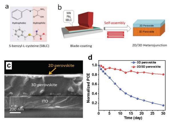
Fig. 7 SBLC molecular structure (a); the blade-coating of the 2D/3D perovskite film schematic (b); SEM surface images of the 2D/3D perovskite film (c); shelf stability of the 3D and 2D/3D heterostructure solar cells stored in ambient air with a relative humidity (RH) of  $50\% \pm 10\%$  (d). This figure has been adapted from ref. 94 with permission from John Wiley and Sons, copyright 2020.
