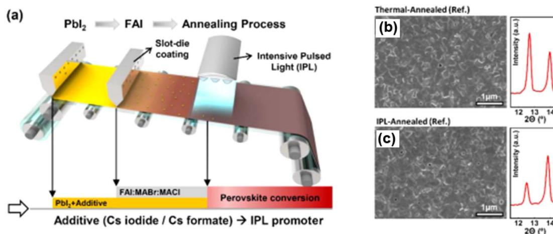
Fig. 8 Schematic representation of the R2R two-step processing method utilizing an IPL treatment (a); FE-SEM and XRD graphs of the perovskite surface (pristine  $\text{PbI}_2$ ) (b); FE-SEM and XRD (pristine  $\text{PbI}_2$ ) analysis of perovskite surfaces treated with IPL (c). This figure has been adapted from ref. 71 with permission from American Chemical Society, copyright 2024.
