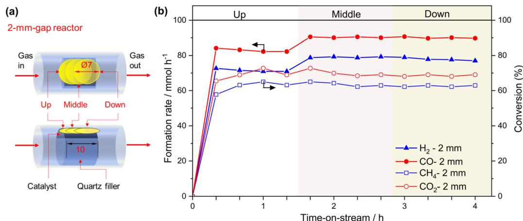
Fig. 6 Effect of the position of the light spot on the photothermal catalytic activity. (a) Schematic representation. (b) Formation rates of H<sub>2</sub> and CO (left-axis) and conversion (right-axis) of CH<sub>4</sub> and CO<sub>2</sub> using the 2-mm-gap reactor. ( $P = 25$  W,  $\Phi = 7$  mm.)
