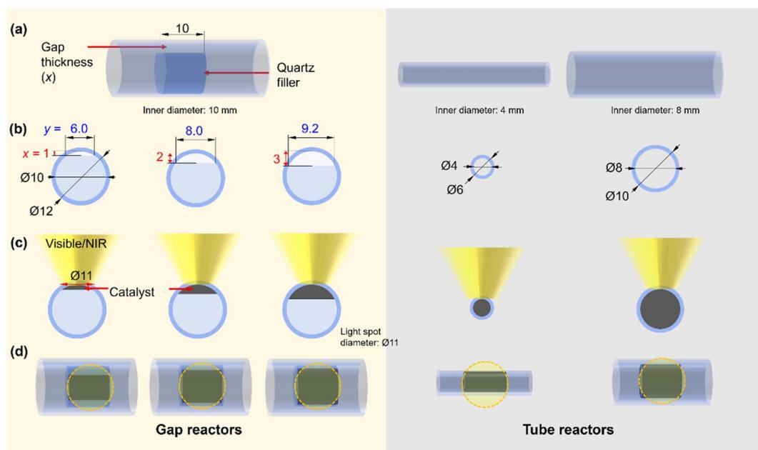
Fig. 1 Schematic representation of the photo-reactors used in this study. (a) Overview. (b) Side view. (c) Side view with catalyst. (d) Top view with catalyst. The light spot diameter of 11 mm  $\Phi$  is used for the representation. Dimensions are in mm.
