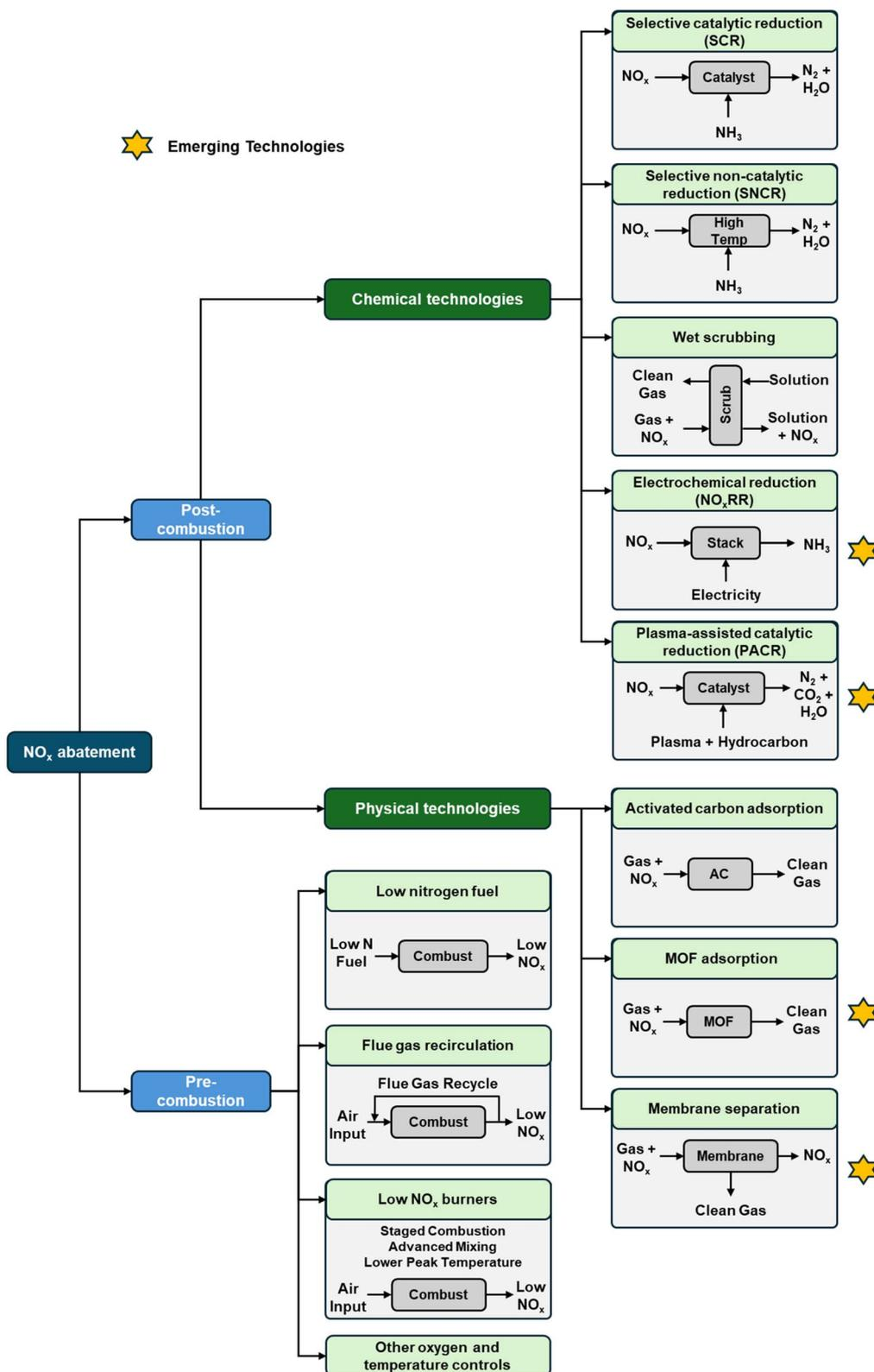
Fig. 3 Simplified schematics for current and emerging NO<sub>x</sub> abatement technologies.
