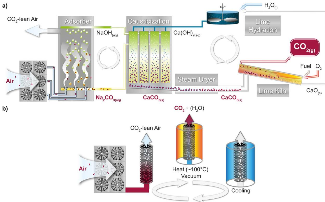
Fig. 4 Schematic representation of DAC technologies. (a) Calcium looping, featuring the chemical reaction between atmospheric  $\text{CO}_2$  and aqueous sodium hydroxide to form sodium carbonate, followed by the calcium cycle, where calcium hydroxide regenerates NaOH via causticization and calcination steps. (b) Amine-based DAC, including the capture of atmospheric  $\text{CO}_2$  in a packed bed of solid amine sorbent, followed by regeneration at elevated temperature and cool-down.
