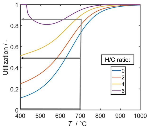
Fig. 5 Carbon formation limit as a function of temperature and utilization of CO<sub>2</sub> and water as well as the H/C ratio. Carbon formation is thermodynamically favored when operating in conditions above the corresponding curve. The methodology for the calculations is given in the ESI.†
