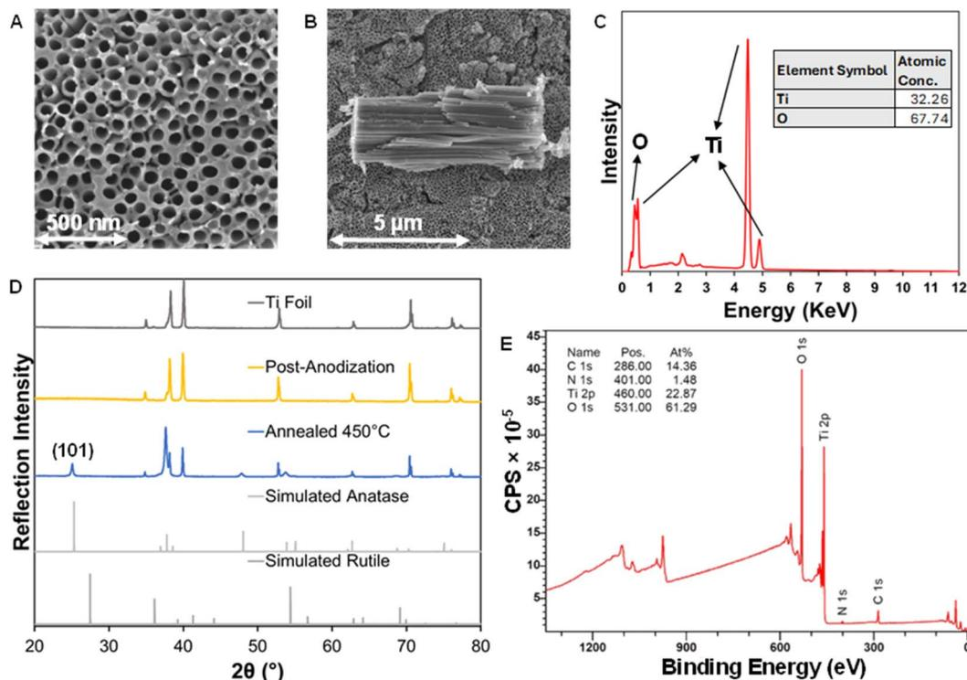
Fig. 3 (A) SEM micrograph of a  $\text{TiO}_2$  NT surface, (B) cross-sectional SEM micrograph of  $\text{TiO}_2$  NTs, (C) EDS elemental analysis of  $\text{TiO}_2$  NTs, (D) PXRD diffractogram of  $\text{TiO}_2$  NTs (simulated anatase AMCSD 0019093 and simulated rutile AMCSD 0001735) and (E) XPS survey of  $\text{TiO}_2$  NTs.
