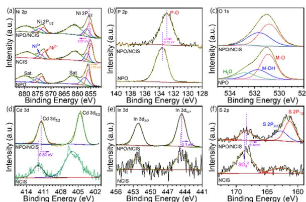
Fig. 2 High-resolution XPS spectra of (a) Ni 2p, (b) P 2p, (c) O 1s, (d) Cd 3d, (e) In 3d and (f) S 2p in NH<sub>4</sub>NiPO<sub>4</sub>·H<sub>2</sub>O, CdIn<sub>2</sub>S<sub>4</sub>/Ni<sub>3</sub>S<sub>2</sub>, and NH<sub>4</sub>-NiPO<sub>4</sub>·H<sub>2</sub>O/CdIn<sub>2</sub>S<sub>4</sub>/Ni<sub>3</sub>S<sub>2</sub> heterostructure.
