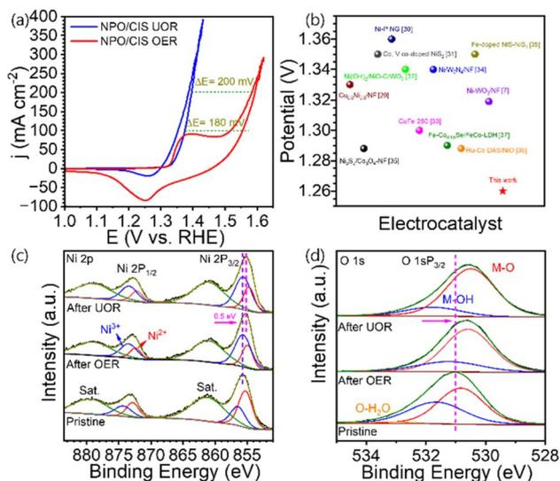
Fig. 5 (a) CV curves of NH<sub>4</sub>NiPO<sub>4</sub>·H<sub>2</sub>O/CdIn<sub>2</sub>S<sub>4</sub>/Ni<sub>3</sub>S<sub>2</sub> heterostructure for OER and UOR at a scan rate of 5 mV s<sup>-1</sup>. (b) Comparison of the UOR activity of the NH<sub>4</sub>NiPO<sub>4</sub>·H<sub>2</sub>O/CdIn<sub>2</sub>S<sub>4</sub>/Ni<sub>3</sub>S<sub>2</sub> heterostructure with various electrocatalysts. High-resolution XPS spectra of (c) Ni 2p and (d) O 1s before and after OER and UOR activity.
