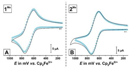
Fig. 3 (A) Overlaid cyclic voltammogram of  $\mathbf{1}^{Me}$  in  $CH_2Cl_2/NBu_4^+$  [BAr $^{F24}$ ] $^-$  (0.1 M, T=293 K ( $\pm 3$  K), v=600 mV s $^{-1}$ , black solid line) and corresponding simulation (blue circles). (B) Overlaid cyclic voltammogram of  $2^{\text{Me}}$  in CH<sub>2</sub>Cl<sub>2</sub>/NBu<sub>4</sub><sup>+</sup> [BAr<sup>F24</sup>]<sup>-</sup> (0.1 M, T = 293 K ( $\pm 3$  K), v = 600 mV s<sup>-1</sup>, black solid line) and corresponding simulation (blue circles).
