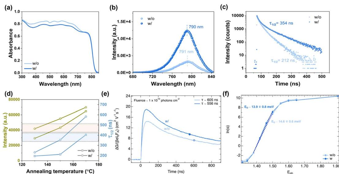
Fig. 2 Opto-electronic properties of the w/o and w/ PbCl<sub>2</sub> samples annealed at 150 °C for 10 minutes. (a) Absorbance spectra, (b) steady state PL, (c) TRPL decay, (d) PL intensity and half-lifetime as a function of annealing temperature; the comparison of PL intensity and half-lifetime is highlighted in light orange and light blue bars, (e) TRMC traces recorded under laser pulses at 650 nm, (f) Urbach energies for w/o and w/PbCl<sub>2</sub> samples.
