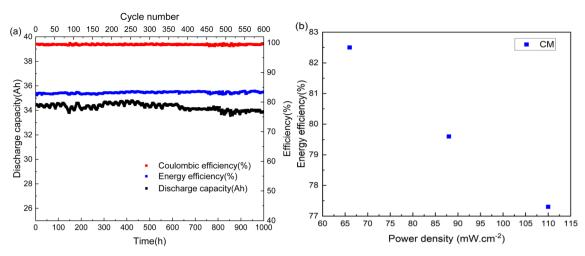
Fig. 4 (a) The electrochemical performance of the 52-stack cell assembled with the CM. (b) The EE for the 52-stack cell assembled with the CM at power densities of 66, 88 and  $110 \text{ mW cm}^{-2}$ .
