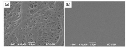
Scanning electron microscopy (SEM) surface images of the (a) HPE membrane and (b) MTCP-50 AEM. Scale bar: 0.5 µm.
