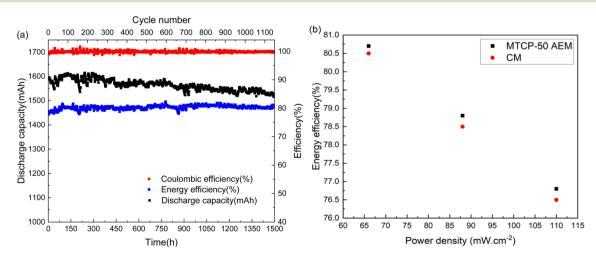
Fig. 3 (a) The electrochemical performance of the single cell assembled with the CM. (b) The EE for the MTCP-50 AEM and CM at power densities of 66, 88 and 110 mW cm<sup>-2</sup> in a single cell.
