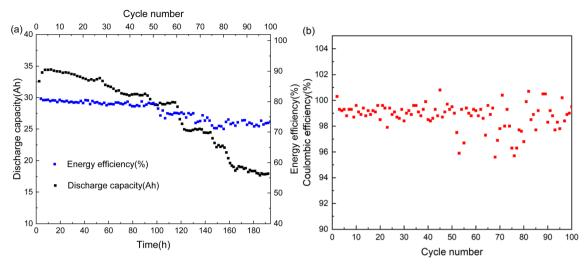
(a) The discharge capacity, EE and (b) CE of the 52-stack cell assembled with the MTCP-50 AEMs.
