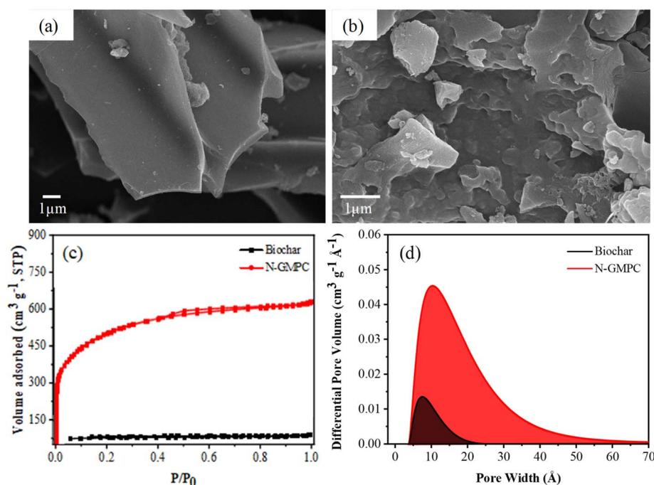
Fig. 1 SEM morphologies of (a) biochar (*Acacia confusa*) and (b) N-GMPC; and (c) N<sub>2</sub> adsorption–desorption isotherms and (d) pore size distribution curves of biochar and N-GMPC.
