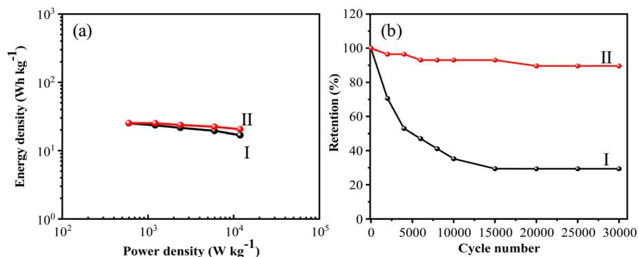
Fig. 10 (a) Ragone plots and (b) cycling stability of CPC (i) and N-GMPC (ii) during 30 000 charge-discharge cycles at a current density of  $10 \text{ mA cm}^{-2}$  (approximately  $4.4 \text{ A g}^{-1}$ ).
