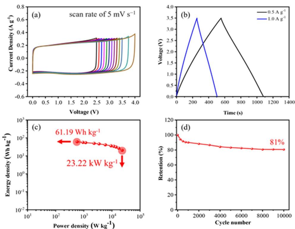
Fig. 11 Electrochemical performance of N-GMPC in 1.0 M SBPBF<sub>4</sub>/ADN electrolyte during 10 000 cycles at a current density of  $1.0 \text{ A g}^{-1}$ . (a) CV curves. (b) GCD curves. (c) Ragone plot. (d) Cycling stability.
