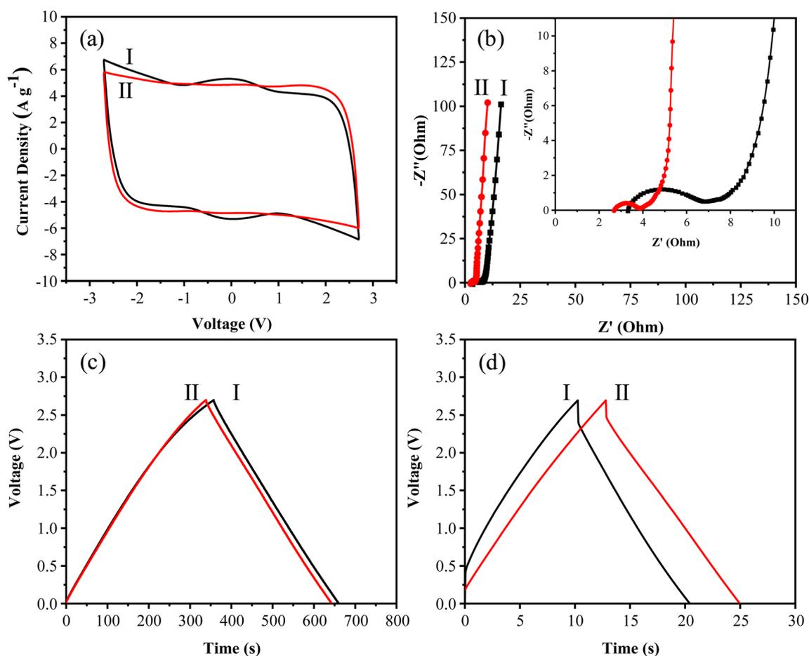
Fig. 8 Electrochemical performance of CPC (I) and N-GMPC (II) symmetric supercapacitors in  $1.0 \text{ M TEABF}_4/\text{PC}$  electrolyte. (a) CV curves at a scan rate of  $200 \text{ mV s}^{-1}$ . (b) EIS spectra. (c) GCD curves at a current density of  $1 \text{ mA cm}^{-2}$ . (d) GCD curves at a current density of  $20 \text{ mA cm}^{-2}$ .
