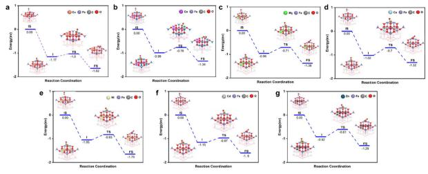
Fig. 4 The reaction process of AFe<sub>2</sub>O<sub>4</sub> spinel with CO. (a) A = Cu. (b) A = Co. (c) A = Mq. (d) A = Ca. (e) A = Ni. (f) A = Cd. (g) A = Zn.
