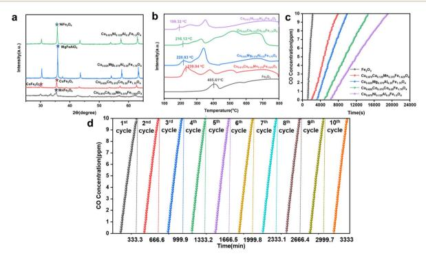
Fig. 10 Low concentration CO chemical looping argon purification experiment test. (a) XRD plots of the OCs. (b) H<sub>2</sub>-TPR test plot for OCs. (c) CO removal performance at 500 °C and 100PPM CO concentration. (d) Stability of  $Cu_{0.875}Ni_{0.125}Al_{0.5}Fe_{1.5}O_4$  at 10 cycles.
