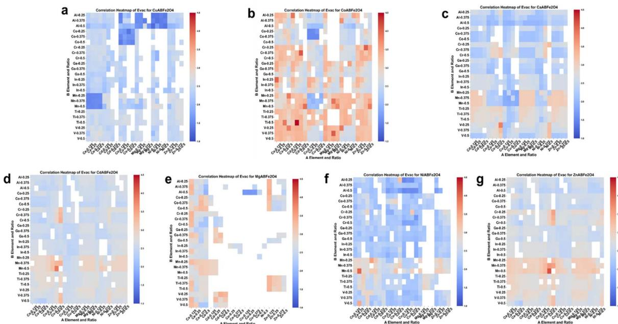
Fig. 9  $E_{\text{vac}}$  heat map of 4375 group OCs. (a)  $\text{Cu}_2\text{BFeO}_4$ . (b)  $\text{Co}_2\text{BFeO}_4$ . (c)  $\text{Ca}_2\text{BFeO}_4$ . (d)  $\text{Cd}_2\text{BFeO}_4$ . (e)  $\text{Mg}_2\text{BFeO}_4$ . (f)  $\text{Ni}_2\text{BFeO}_4$ . (g)  $\text{Zn}_2\text{BFeO}_4$ . White filled sections represent OCs that have been excluded by screening.
