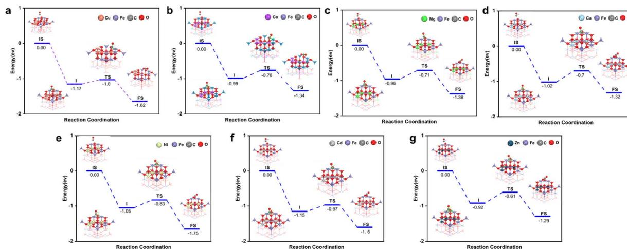
Fig. 4 The reaction process of AFe<sub>2</sub>O<sub>4</sub> spinel with CO. (a) A = Cu. (b) A = Co. (c) A = Mg. (d) A = Ca. (e) A = Ni. (f) A = Cd. (g) A = Zn.
