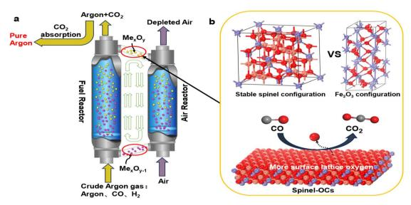
Fig. 1 Chemical looping argon purification principle. (a) Schematic of the chemical looping argon purification process. (b) Structure and reactivity in a conventional oxygen carrier vs. spinel oxygen carrier.
