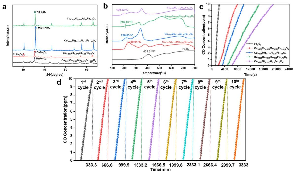
Fig. 10 Low concentration CO chemical looping argon purification experiment test. (a) XRD plots of the OCs. (b)  $\text{H}_2$ -TPR test plot for OCs. (c) CO removal performance at 500 °C and 100PPM CO concentration. (d) Stability of  $\text{Cu}_{0.875}\text{Ni}_{0.125}\text{Al}_{0.5}\text{Fe}_{1.5}\text{O}_4$  at 10 cycles.
