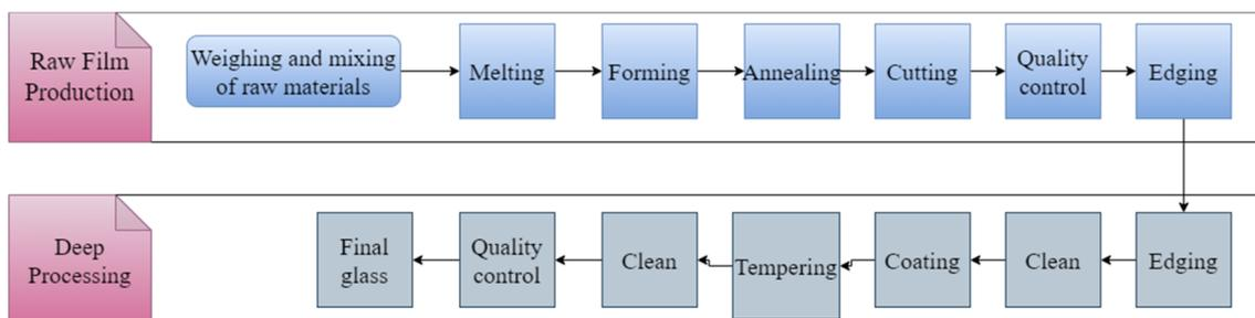
Fig. 1 PV glass production process.<sup>36</sup>
