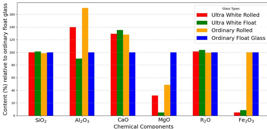
Fig. 2 Chemical component of PV glass compared to ordinary float glass ("R<sub>2</sub>O" stands for alkali oxide).<sup>36</sup>
