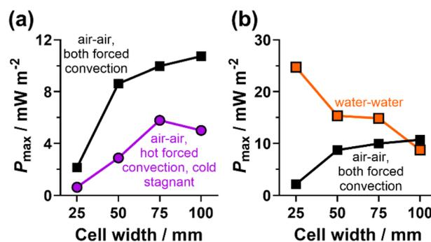
**Fig. 5** Showing  $P_{\text{max}}$  for various cells widths comparing (a) air–air setup with different convection at the colder electrode, and (b) comparing the air–air setup vs. water–water. All other conditions as per Fig. 2 and 4.
