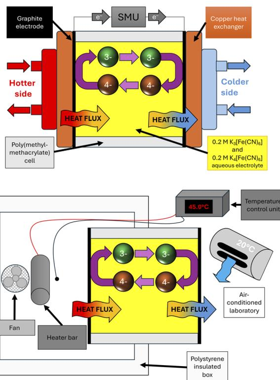
Fig. 1 Annotated cartoons of the (top) water–water thermogalvanic set-up and (bottom) air–air thermogalvanic set-up. Photographs of the setup can be found in the ESI.†
