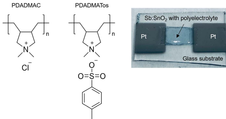
Fig. 1 Chemical formula of PDADMAC and PDADMATos and a photograph of the Sb:SnO 2 /PDADMAX system.
