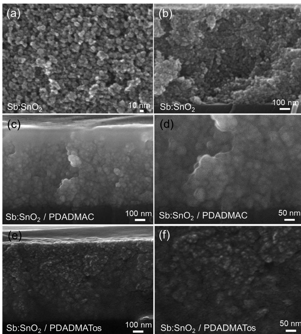
Fig. 4 (a) Top and (b) cross-sectional SEM images of an Sb:SnO<sub>2</sub> film without polyelectrolyte added. Cross-sectional SEM images of Sb:SnO<sub>2</sub> films after addition of (c and d) PDAMAC and (e and f) PDADMATos.
