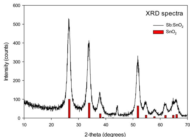
Fig. 3 X-ray diffraction pattern of the Sb:SnO<sub>2</sub> film.
