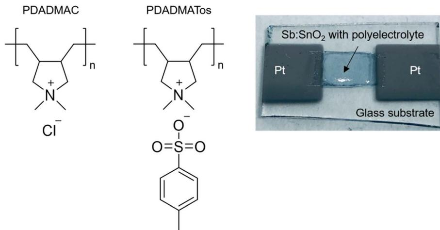
Fig. 1 Chemical formula of PDADMAC and PDADMATos and a photograph of the Sb:SnO<sub>2</sub>/PDADMAX system.
