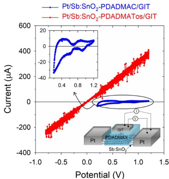
Fig. 6 Cyclic voltammetry experiments at  $5 \text{ mV s}^{-1}$  for Sb:SnO<sub>2</sub> films with PDADMAC (blue) and PDADMATos (red) polyelectrolytes added. The inset shows a scheme of the system measured and how the electrical contacts were established.
