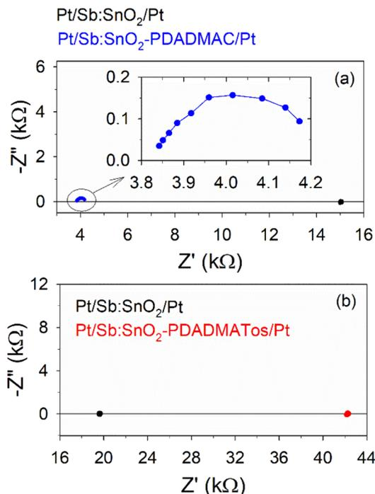
Fig. 5 Impedance spectroscopy carried out at  $\Delta T = 5$  K for the Sb:SnO<sub>2</sub> film before and after the deposition of (a) PDADMAC (sample 1-PDADMAC) and (b) PDADMATos (sample 1-PDADMATos).
