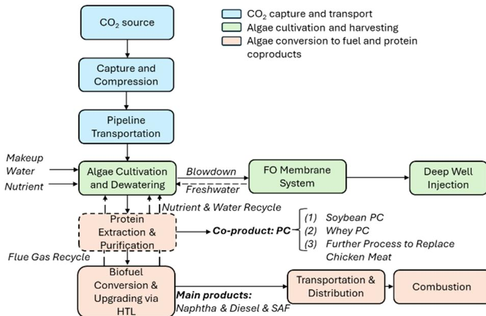
Fig. 1 System boundary flow diagram (dashed box: the protein extraction and purification process applies only to cases involving fuel and protein coproduction).
