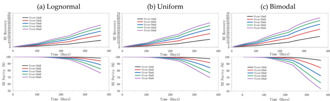
Fig. 8 Hydrogen recovery and purity under different mean permeabilities using different distributions (a) lognormal distribution, (b) uniform distribution, and (c) bimodal distribution in the hydrogen production phase.
