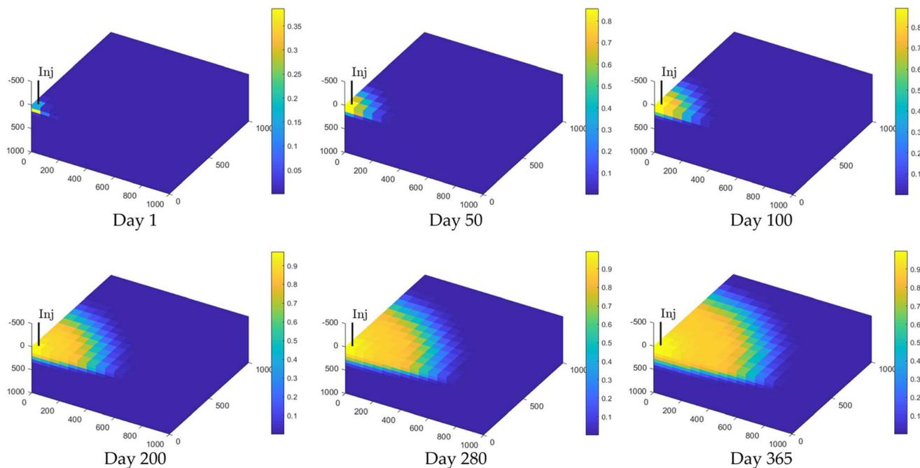
Fig. 4 Reservoir hydrogen concentration distribution on days 1, 50, 100, 200, 280, and 365 during the hydrogen injection phase.
