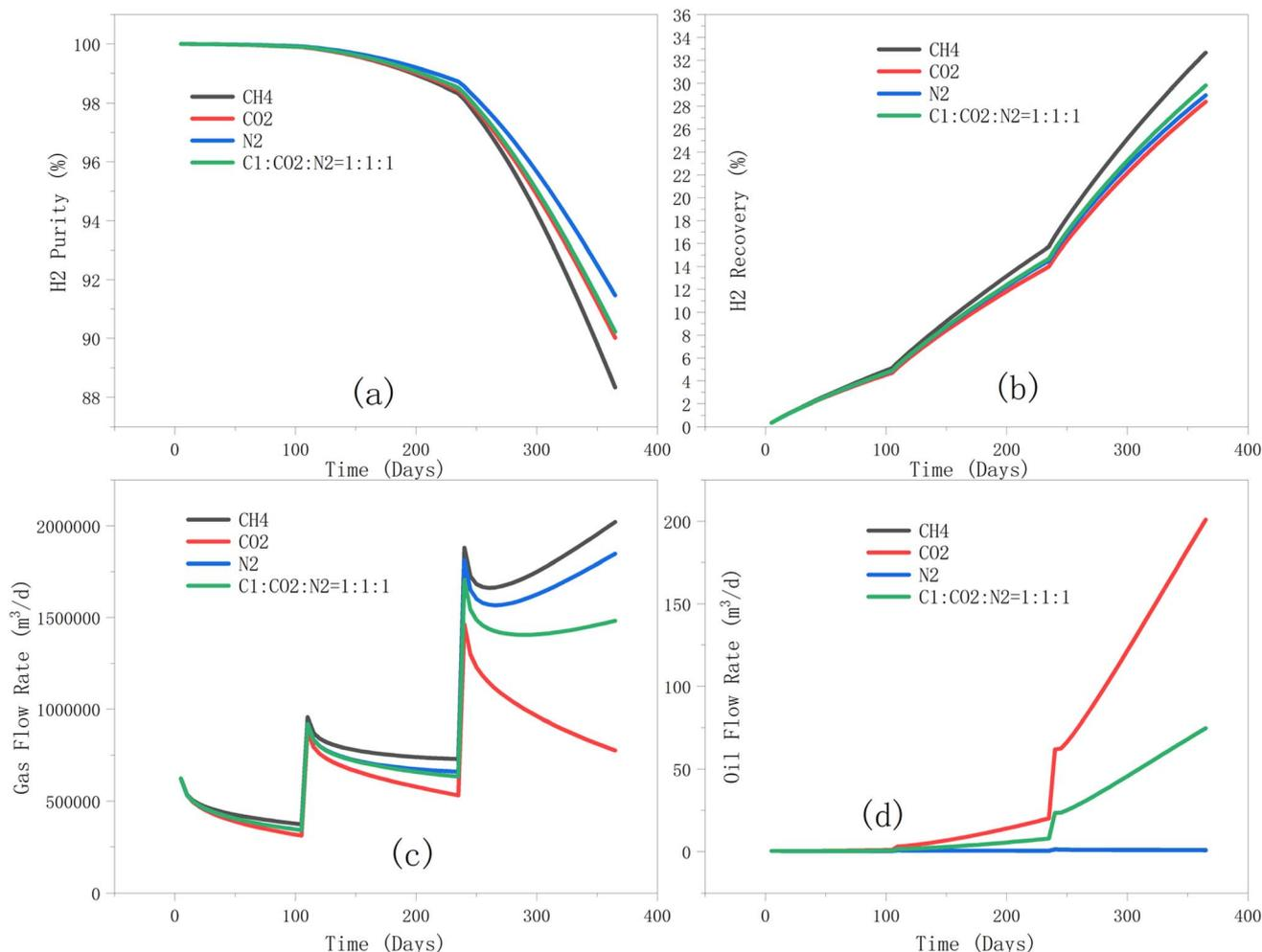
Fig. 17 Impact of cushion gas type on (a) hydrogen purity; (b) hydrogen recovery; (c) gas flow rate; and (d) oil flow rate during the production phase.
