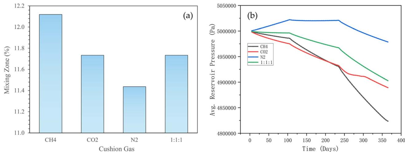
Fig. 18 Effect of cushion gas on (a) the mixing zone during the hydrogen injection phase; and (b) the average reservoir pressure during hydrogen production (1 bar  $\equiv$  100 000 Pa).
