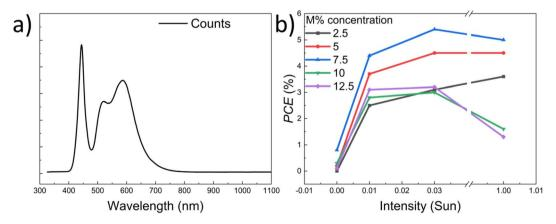
Fig. 4 (a) Spectrum of the LED used to test indoor PV performance and (b) the corresponding PCE under different light intensities for FASI with different mol% concentration of MASnClz.
