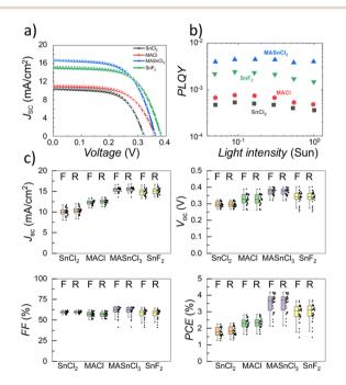
Fig. 3 Comparison of the performance of  $FASnI_3$  devices printed with the four additives studied,  $SnCl_2$ , MACl,  $MASnCl_3$ ,  $SnF_2$ . (a) JV scans; (b) light-intensity-dependent photoluminescence quantum yield of each sample (full device stack); (c) JV performance distribution (F for forward and R for reverse scans) of each sample.
