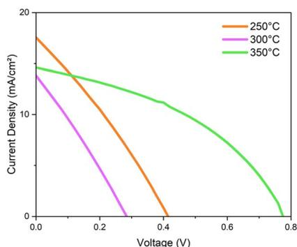
**Fig. 4** Illuminated JV curves for the devices based on CZTS NPs HTM annealed at 350 °C, 300 °C and 250 °C.
