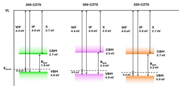
Fig. 3 Electronic structures for the 350-CZTS, 300-CZTS and 250-CZTS layers. The distances of VBM from  $E_{\text{Fermi}}$  were obtained thanks to XPS analysis; WFs were extrapolated from UPS spectra; and the  $B_{\text{gap}}$  values were obtained through UV-vis measurements. All the other values have been calculated.
