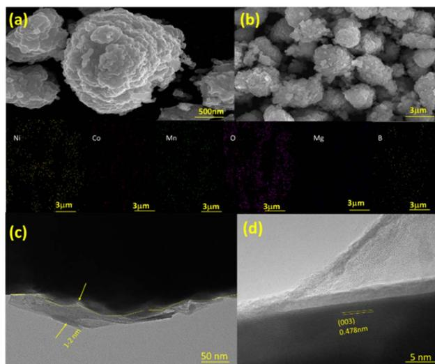
Fig. 2 (a & b) SEM and EDX images of NCM-622 and BM NCM-622. (c & d) HR-TEM images of BM NCM-622.
