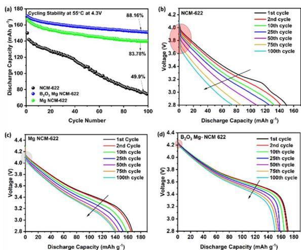
Fig. 5 (a) Cycling stability studies upon cycling at 1C at 55 °C (2.8 to 4.3 V) and (b to d) average discharge voltage graphs for all the cathodes.
