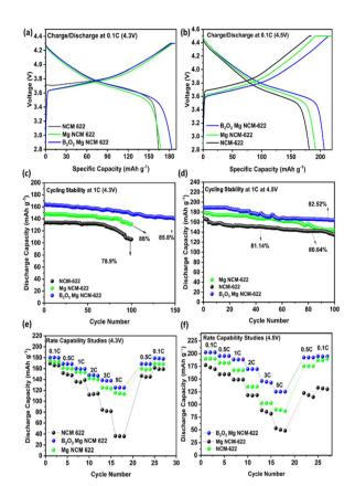
Fig. 4 (a & b) Initial charge/discharge graph of all three cathodes at 4.3 V and 4.5 V, (c & d) cycling study graphs of all the cathodes at 4.3 V and 4.5 V, and (e & f) rate capability studies for all the cathodes at 4.3 V 845V
