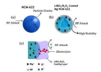
Fig. 8 (a) Bare NCM-622, (b) dual-modified NCM-622 & (c) mechanism of surface protection using the hybrid layer.
