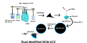
Scheme 1 Synthesis of Mg NCM-622 by using a CSTR and wet chemical coating of the LiBO<sub>2</sub>/B<sub>2</sub>O<sub>3</sub> layer on Mg NCM-622.
