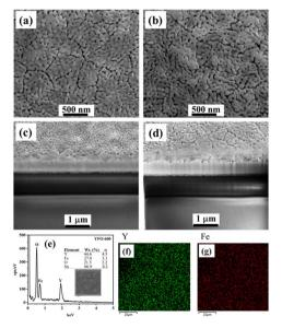
Fig. 2 Top view (a) and cross-sectional (c) SEM images of the o-YFO film; SEM images of top view (b) and cross-section (d) of the o-YFO film after the hydrogen evolution reaction. EDX spectrum (e) and elemental mapping of Y (f) and Fe (g) of the o-YFO film.
