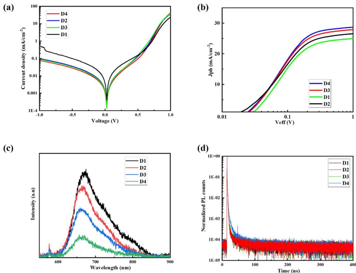
Fig. 3 (a) Dark current–voltage characteristics of the fabricated solar cells for CN and DIB-based devices. (b) Variations of photocurrent ( $J_{ph}$ ) with an effective bias voltage ( $V_{eff}$ ) in OSCs for CN and DIB-based devices with different ETL. (c and d) PL and TRPL spectra for CN and DIB-based devices with different ETL.
