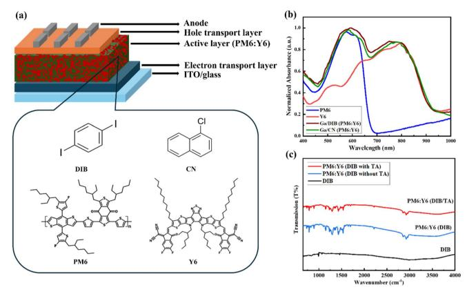
Fig. 1 (a) Schematic diagram of the inverted device structure of non-fullerene OSCs, and chemical structures of additives, donor materials, and acceptor materials (b) absorption spectra of PM6, Y6, Ga/DIB (PM6:Y6) and Ga/CN (PM6:Y6). (c) Fourier transform infrared spectroscopy (FTIR) transmission spectra of DIB with and without thermal annealing
