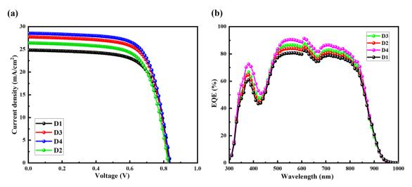
Fig. 2 (a) Current density versus voltage (J-V) characteristics of the best-performed devices based on PM6:Y6 with solvent additive CN and solid additive DIB. (b) EQE spectra of PM6:Y6 with solvent additive CN and solid additive DIB [here, ZnO as an electron transport layer (ETL) with the addition of the solvent additive CN and the solid additive DIB, referred to as devices D1 and D3. Also, devices D2 and D4 correspond to GZO ETL with the addition of CN and DIB, respectively].
