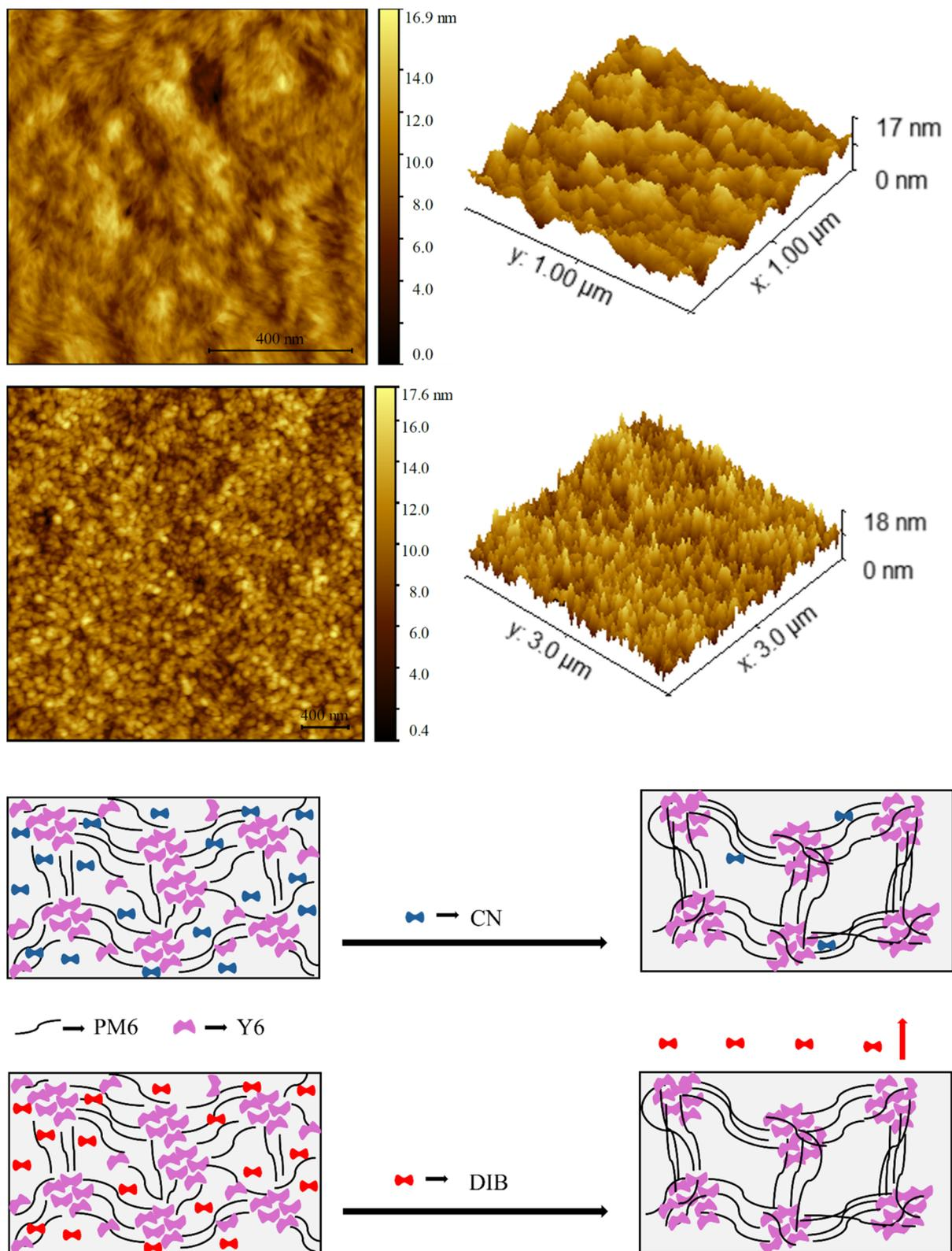
Fig. 5 Atomic force microscopy (AFM) images of PM6:Y6 with solvent additive CN and solid additive DIB-based films respectively.
