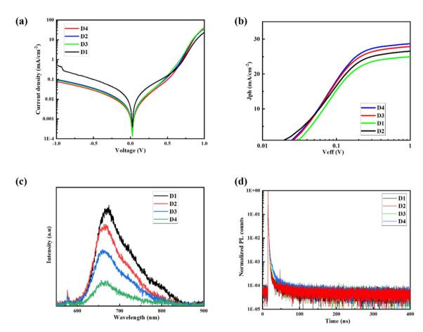
Fig. 3 (a) Dark current-voltage characteristics of the fabricated solar cells for CN and DIB-based devices. (b) Variations of photocurrent  $(J_{ob})$ with an effective bias voltage ( $V_{eff}$ ) in OSCs for CN and DIB-based devices with different ETL. (c and d) PL and TRPL spectra for CN and DIB-based devices with different ETL.
