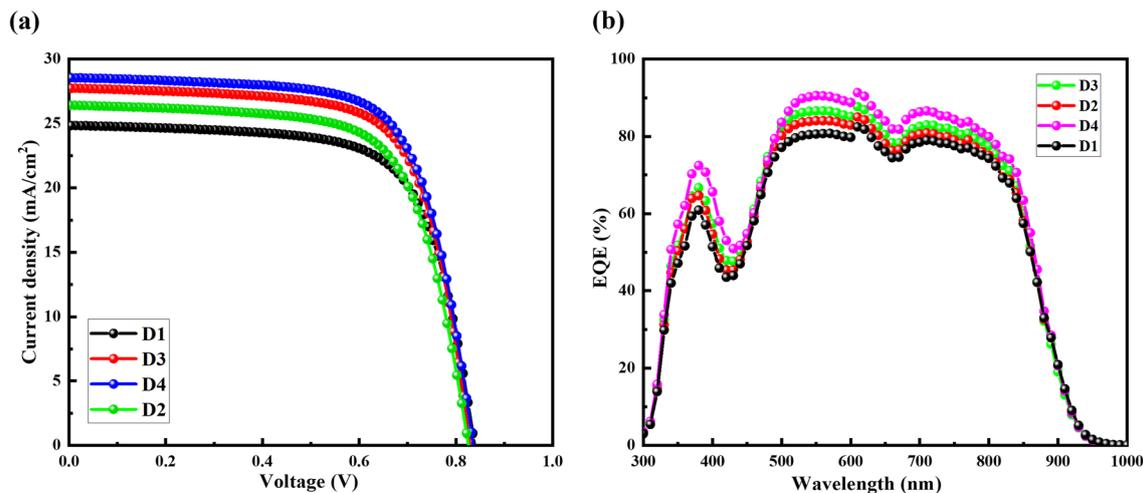
Fig. 2 (a) Current density versus voltage ( $J$ - $V$ ) characteristics of the best-performed devices based on PM6:Y6 with solvent additive CN and solid additive DIB. (b) EQE spectra of PM6:Y6 with solvent additive CN and solid additive DIB [here, ZnO as an electron transport layer (ETL) with the addition of the solvent additive CN and the solid additive DIB, referred to as devices D1 and D3. Also, devices D2 and D4 correspond to GZO ETL with the addition of CN and DIB, respectively].
