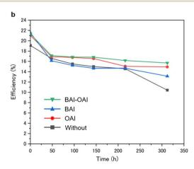
Fig. 3 (a) I-V curves of devices fabricated under each condition. (b) Plots of light durability tests at 40% RH and 30 °C. Green, blue, red and black lines show the device condition with BAI-OAI, BAI, OAI and without passivation, respectively.
