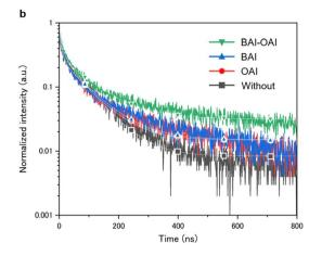
Fig. 2 (a) Steady-state photoluminescence (PL) spectra and (b) time-resolved photoluminescence (TRPL) spectra of devices with different passivation materials on the perovskite layer.
