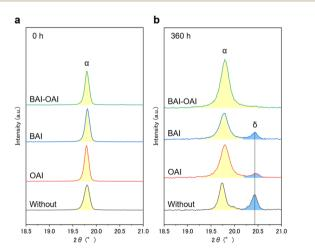
Magnified XRD spectra of each condition (a) before light irradiation and (b) exposed under a solar simulator for 360 hours.
