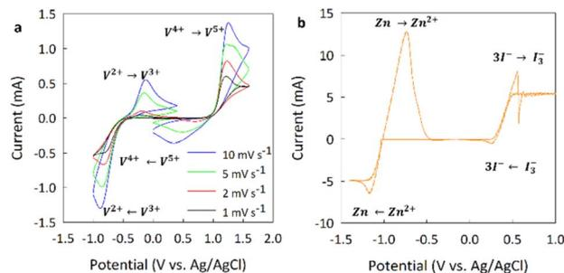
Fig. 4 Electrochemical characterization of redox electrolytes on glassy carbon electrodes. Cyclic voltammograms of (a) vanadium electrolyte at varying scan rates and (b) zinc iodine electrolyte at a scan rate of  $10 \text{ mV s}^{-1}$ .
