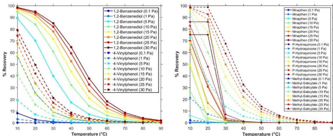
Fig. 6 (left) The % recovery of rice husk (levoglucosan, 1,2-benzenediol, and 4-vinylphenol) and (right) forestry residue (mnapthen, *p*-hydroquinone, and methyl-salicylate) models isolated compounds at varying temperatures and pressures.
