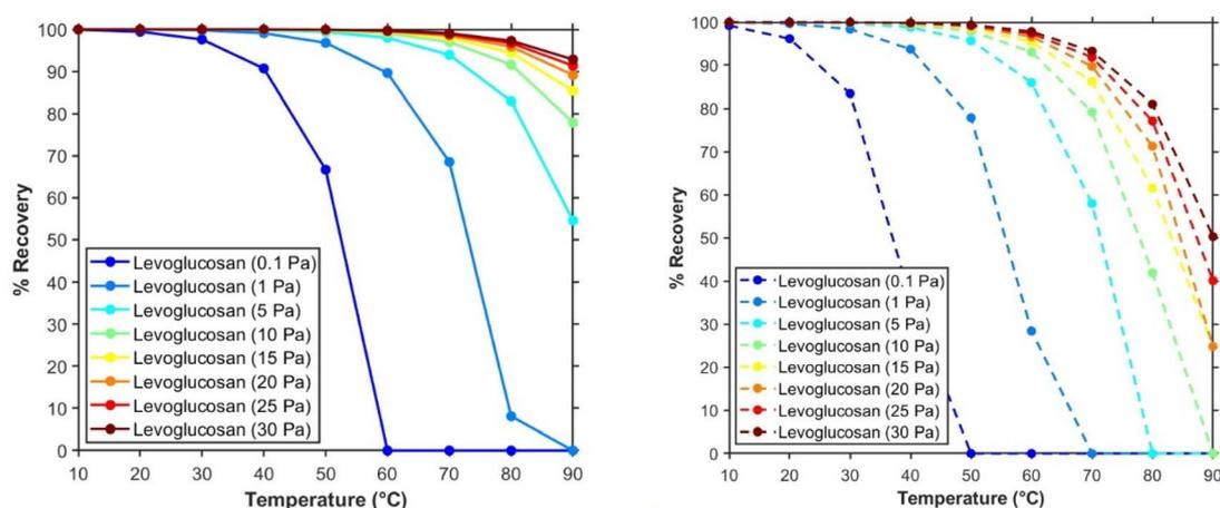
Fig. 5 The % recovery of levoglucosan at varying temperatures and pressures for (left) rice husk and (right) forestry residue models.
