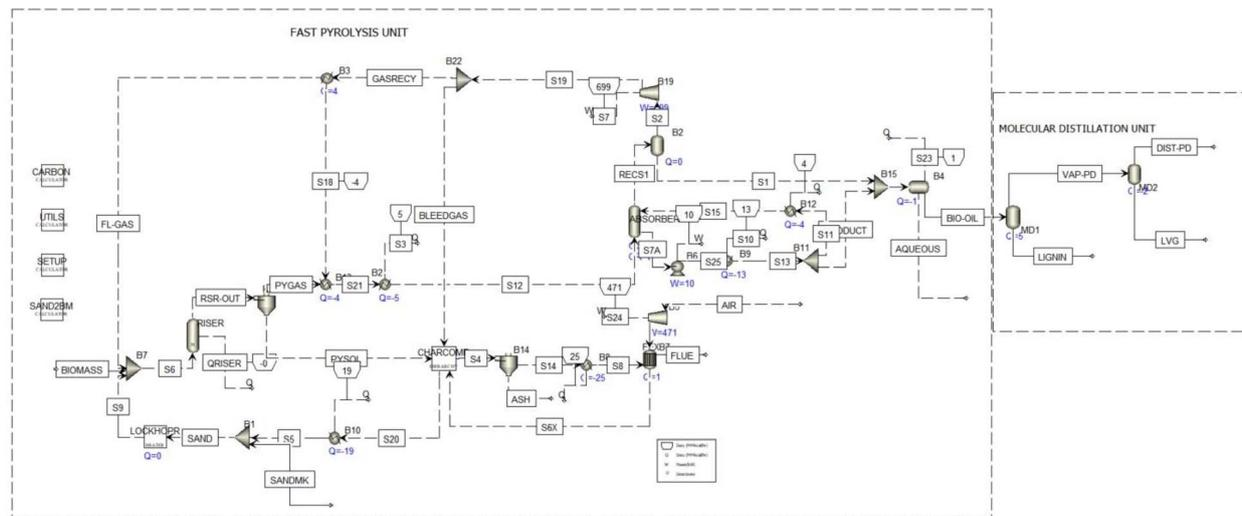
Fig. 1 Overview of the flowsheet for the integration of molecular distillation with fast pyrolysis of biomass.
