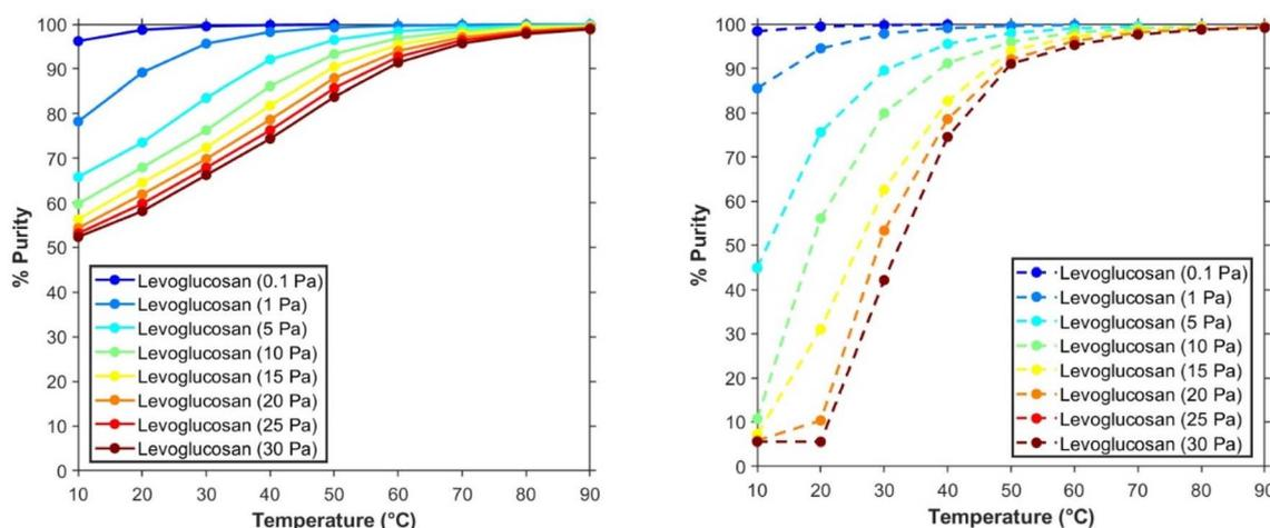
Fig. 7 The % Purity of levoglucosan in the LVG stream of MD2 at varying temperatures and pressure for (left) rice husk and (right) forestry residue model.
