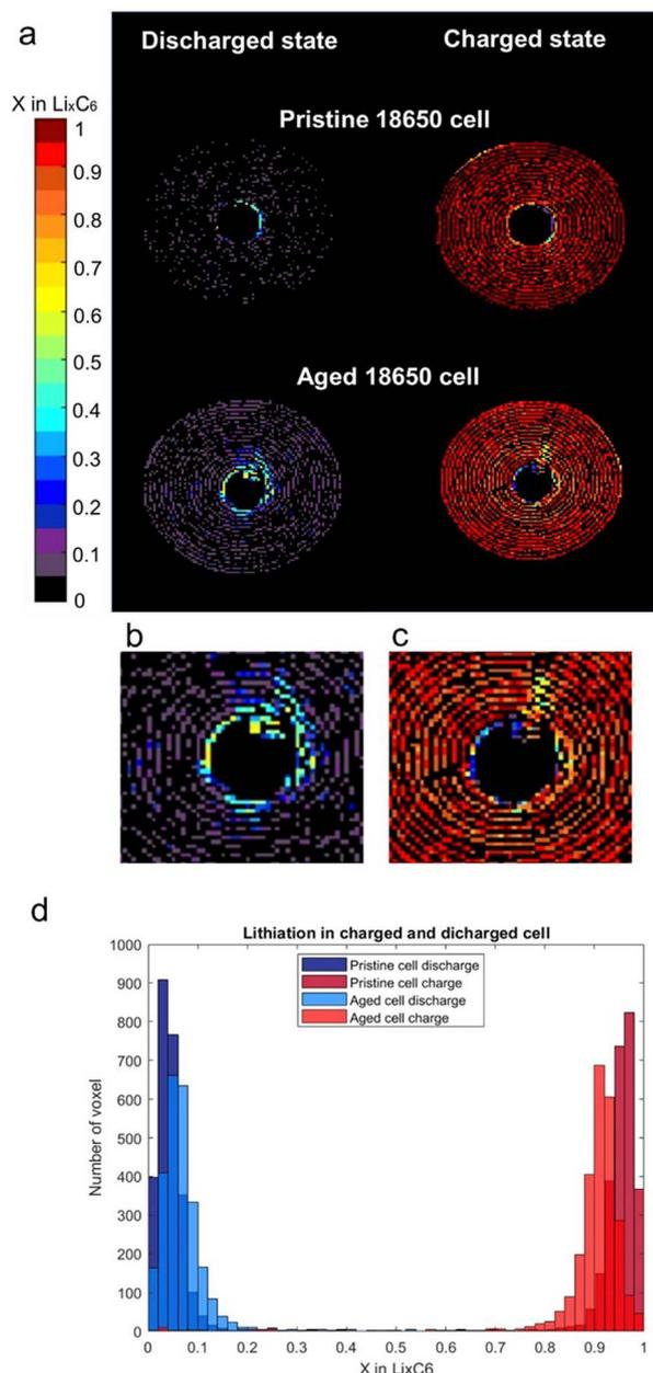
Fig. 4 (a) Comparison between pristine and aged cell at charged and discharged state. The  $x$  in  $\text{Li}_x\text{C}_6$  is plotted as colour bar across the volume area. (b) Zoom of aged discharged cell. (c) Zoom of aged charged cell. (d) Number of voxels vs.  $x$  value in  $\text{Li}_x\text{C}_6$  at discharged and full charged state of aged cell. (e) Damaged zone extended into the volume from the centre, probably derived from the spiral collapsing.
