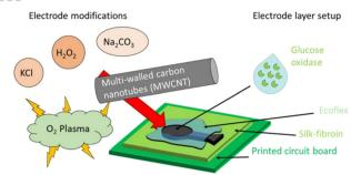
Modification of a bioabsorbable carbon electrode on silk-fibroin carriers: setting the composition and adjustment of the working potential
