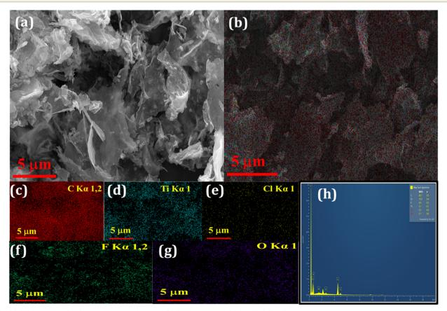
Fig. 2 (a) FESEM image, (b-g) elemental mappings and (h) EDX analysis of COOH-Ti<sub>3</sub>C<sub>2</sub>T<sub>x</sub> NSs.
