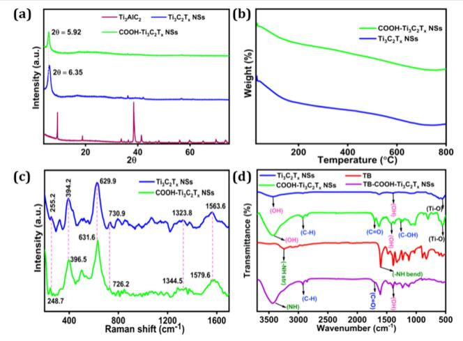
Fig. 3 (a) XRD patterns of Ti<sub>3</sub>AlC<sub>2</sub>, Ti<sub>3</sub>C<sub>2</sub>T<sub>x</sub> NSs and COOH-Ti<sub>3</sub>C<sub>2</sub>T<sub>x</sub> NSs. (b) TGA curves of Ti<sub>3</sub>C<sub>2</sub>T<sub>x</sub> NSs and COOH-Ti<sub>3</sub>C<sub>2</sub>T<sub>x</sub> NSs. (c) Raman spectra of  $Ti_3C_2T_x$  NSs and COOH- $Ti_3C_2T_x$  NSs. (d) FTIR spectra of  $Ti_3C_2T_x$  NSs, COOH- $Ti_3C_2T_x$  NSs, TB and TB/COOH- $Ti_3C_2T_x$  NSs.
