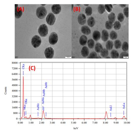
Fig. 5 (A) TEM image of GNPs, (B) TEM image folate-conjugated GNPs, and (C) EDS of folate-conjugated GNPs.
