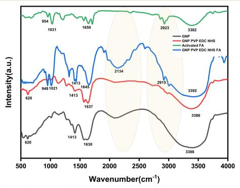
Fig. 4 FTIR spectra of GNP and folate-conjugated GNPs.
