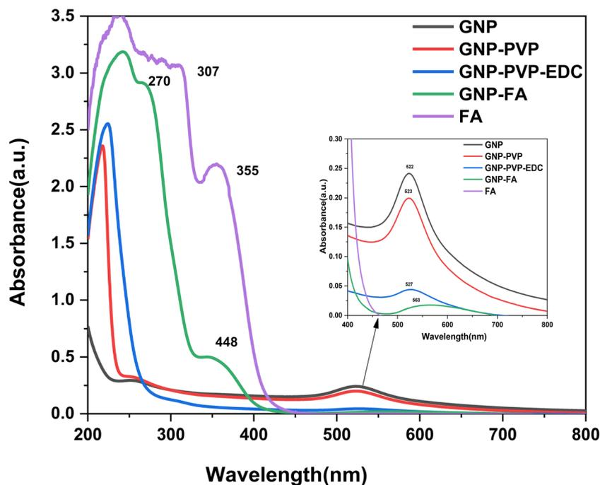
Fig. 3 UV-visible spectra of GNP and folate-conjugated GNPs.
