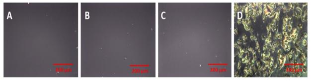
Fig. 6 Optical images (under crossed polarizer) of LC cells in the presence of different concentrations of folate@GNP (A)  $1~\mu g~mL^{-1}$ , (B)  $2~\mu g~mL^{-1}$ (C) 5  $\mu g$  mL<sup>-1</sup> and (D) 10  $\mu g$  mL<sup>-1</sup>.
