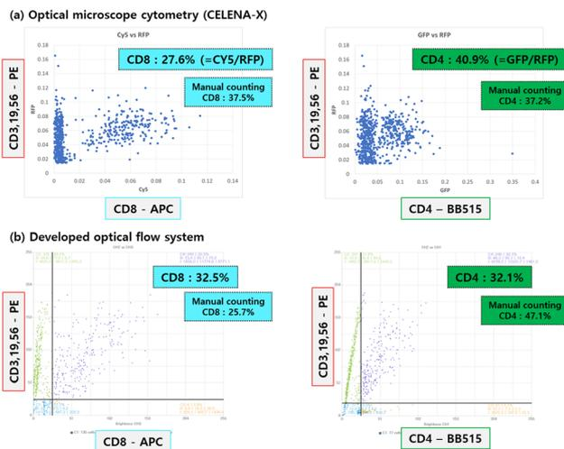
**Fig. 4** Classification results of CD4 and CD8 cells. (a) Results obtained using a commercial optical microscopy-based flow cytometry and (b) the corresponding results obtained from the developed optical flow system.
