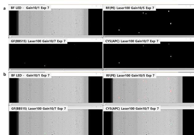
**Fig. 3** (a) Bright field and fluorescence images of flowing WBCs, together with their corresponding binary images for each fluorescence label (PE, BB515, and Cy5). (b) Automatically generated overlaid images showing WBCs with distinct colors according to their antibody-specific labeling.
