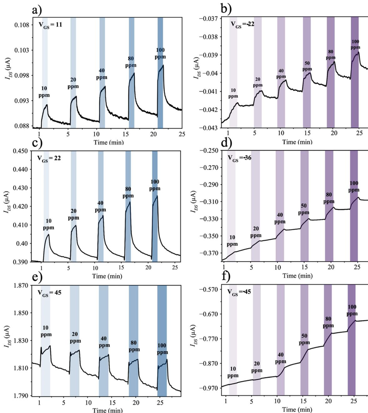
**Fig. 4** Response of OTFT sensors under successive exposure of  $\text{NH}_3$  for 1 min and recovery under synthetic air for 4 min in the range of  $\text{NH}_3$  concentration from 10–100 ppm in dry air and 20–22°C at different  $V_{\text{GS}}$ . a), c) and e)  $\text{F}_{16}\text{CuPc}$  OTFT and b), d) and f)  $\text{CuPc}$  OTFT. For  $\text{F}_{16}\text{CuPc}$ , a  $V_{\text{DS}} = 45$  V was used for all the measurements and for  $\text{CuPc}$ ,  $V_{\text{DS}} = -45$  V.
