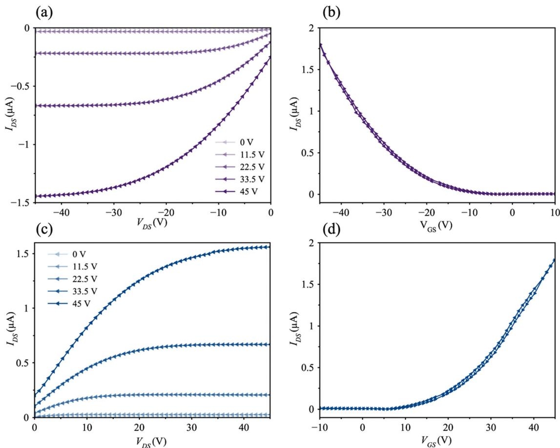
Fig. 2 Output and transfer characteristics of  $CuPc$  (a and b) and  $F_{16}CuPc$  (c and d) OTFTs. Transfer curves were measured at  $V_{DS} = -45$  V for  $CuPc$  and  $V_{DS} = 45$  V for  $F_{16}CuPc$ , with  $V_{GS}$  swept from 10 to  $-45$  V and  $-10$  to 45 V, respectively. Output curves were measured at  $V_{GS}$  of (0,  $-11.5$ ,  $-22.5$ ,  $-33.5$  and  $-45$ ) for  $CuPc$  and (0, 11.5, 22.5, 33.5 and  $-45$ ) for  $F_{16}CuPc$ .
