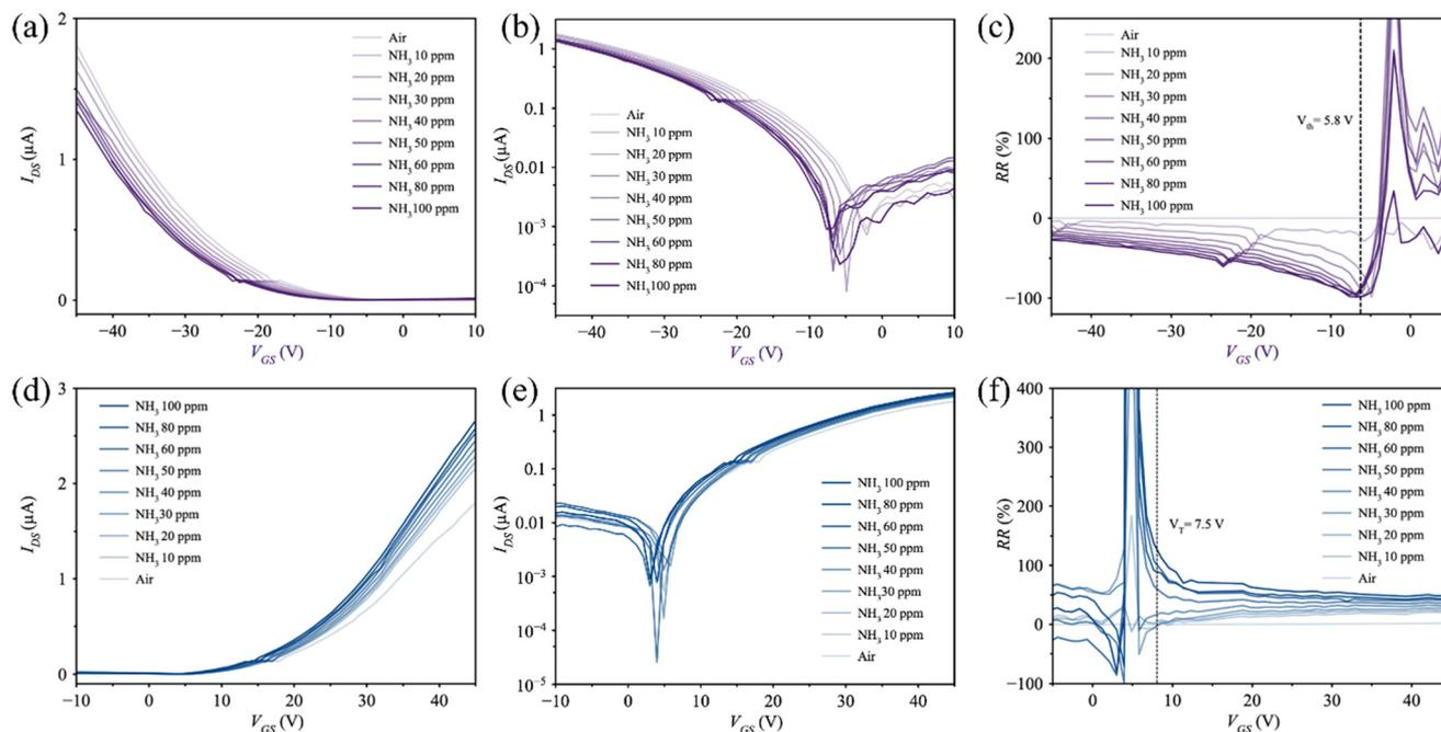
**Fig. 3** Transfer curves at different ammonia concentrations of CuPc: a) linear plot and b) log plot, and F<sub>16</sub>CuPc: d) linear plot and e) log plot. The relative response as a function of gate voltage for c) CuPc and f) F<sub>16</sub>CuPc OTFTs as a function of ammonia concentrations.
