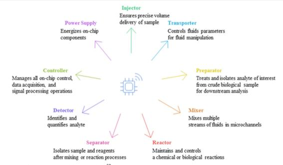
Fig. 3 Overview of LoC components and their functions. 59
