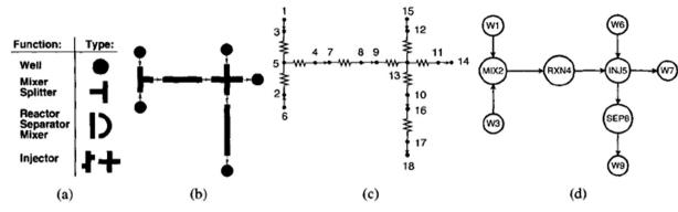
Fig. 2 The LoC simulation process: a) partial library of LoC units, b) channel topology constructed from the library of unit, c) resistor network representation of the channel topology, and d) directed acyclic graph representation of the channel topology. Reproduced from ref. 58 with permission from Elsevier, copyright 2006.
