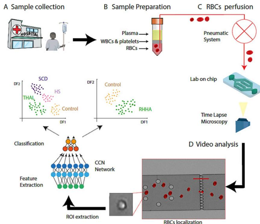
**Fig. 13** Schematic representation of RBC shape analysis. A) Sample collection, B) sample preparation, C) RBC perfusion, and D) video analysis. Reproduced from ref. 112 with permission from *Scientific Reports*, copyright 2021.
