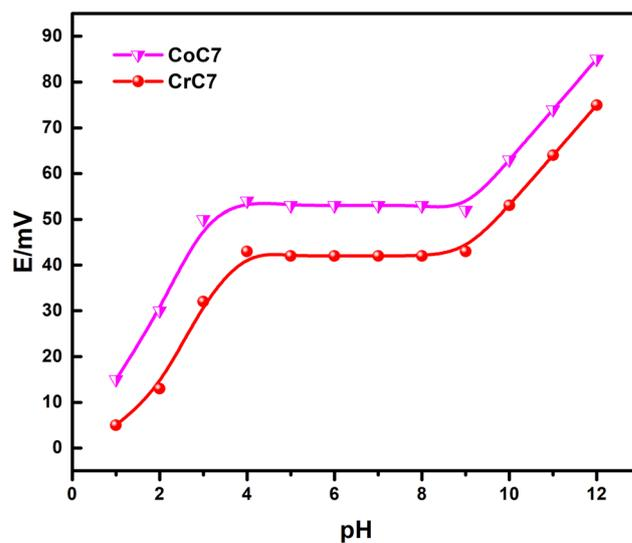
Fig. 5 Effects of pH on the performance of proposed electrode solutions with bromide at a concentration of  $1.0 \times 10^{-2}$  mol L<sup>-1</sup>.
