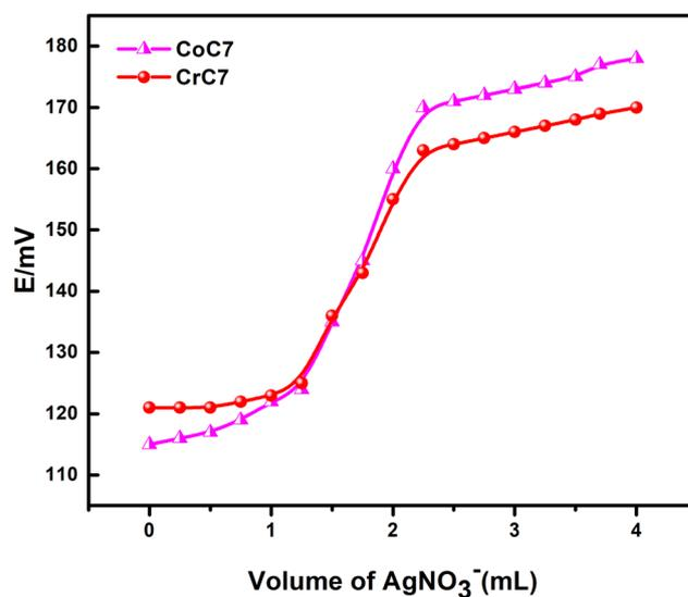
**Fig. 7** Potentiometric titration of 20 mL solution of 1.0 × 10<sup>-2</sup> mol L<sup>-1</sup> NaBr against 1.0 × 10<sup>-1</sup> mol L<sup>-1</sup> AgNO<sub>3</sub> solution.
