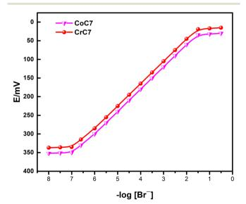
Fig. 4 Calibration curves for the best performing electrodes CoC7 and CrC7.
