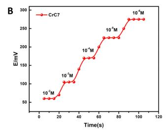
Fig. 6 (A and B) Dynamic response times of CoC7 and CrC7 electrodes.
