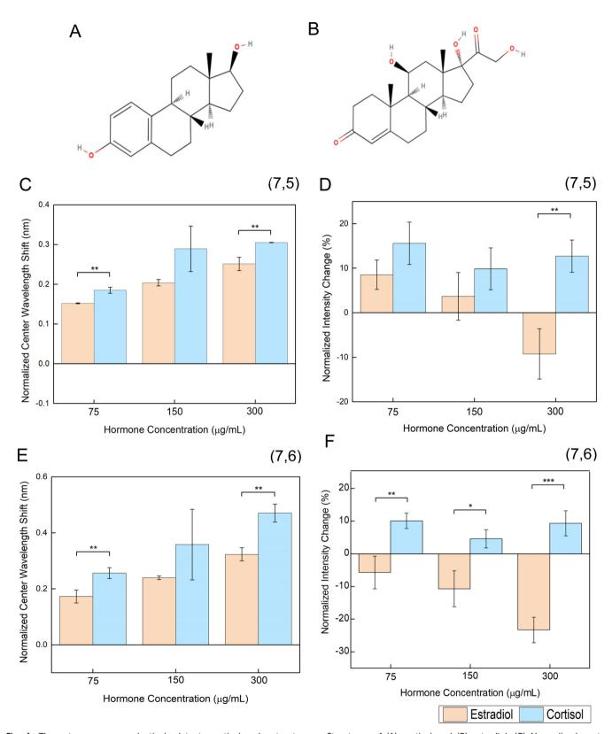
Fig. 4 The aptananosensor selectively detects cortisol and not estrogen. Structures of (A) cortisol and (B) estradiol. (C) Normalized center wavelength shift and (D) intensity change for the (7,5) peak of HiPCO SWCNT-aptamer sensor. (E) Normalized center wavelength shift and (F) intensity change, for the (7,6) peak of HiPCO SWCNT-aptamer sensor. \* = p < 0.05, \*\* = p < 0.01; \*\*\* = p < 0.001.
