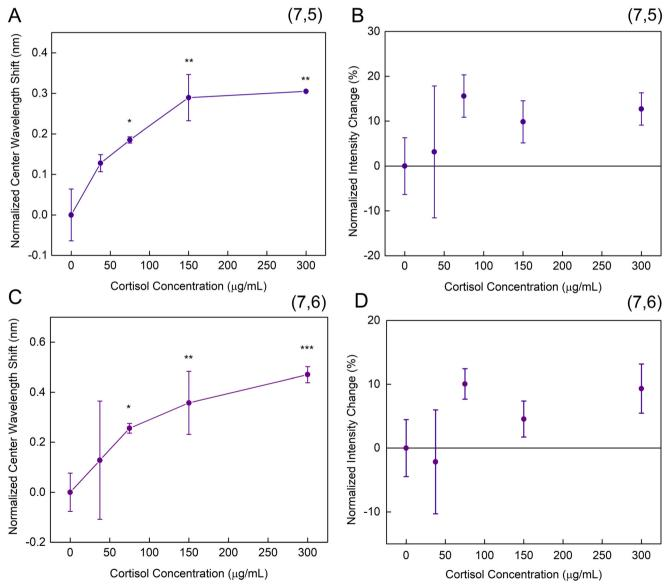
Fig. 2 Dynamic range of aptananosensor response to cortisol. (A) Normalized center wavelength shift and (B) normalized intensity change, in (7,5) SWCNTs peak with increasing cortisol concentration after 3 hours. (C) Normalized center wavelength shift and (D) normalized intensity change, in (7,6) SWCNTs peak with increasing cortisol concentration after 3 hours. \* = p < 0.5, \*\* = p < 0.01, \*\*\* = p < 0.001.
