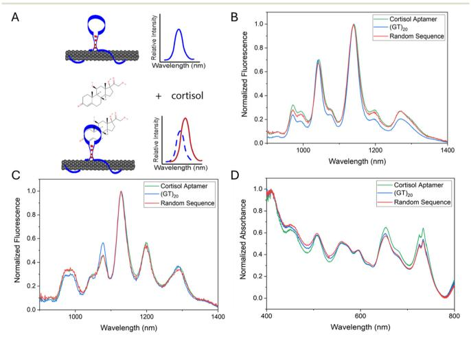
Fig. 1 Cortisol detection strategy and sensor/control characterization. A) A SWCNT-based aptananosensor detection strategy for the stress hormone cortisol. Fluorescence spectra of SWCNT functionalized with cortisol aptamer, (GT)<sub>20</sub> and a random 40mer sequence with laser excitation at (B) 655 nm and (C) 730 nm. (D) UV-vis absorbance spectra of the SWCNT constructs.
