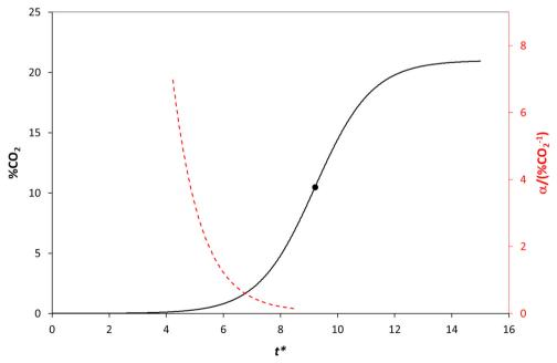
Fig. 2 Plot of  $CO_2$  vs. unitless time parameter  $t^*$ , calculated using eqn (7), assuming  $N_{\text{max}}$  and  $N_0$  are  $10^8$  and  $10^4$  CFU mL<sup>-1</sup>, respectively. The broken red line is a plot of the calculated variation in  $t_{TT}^*$  for a series of CO<sub>2</sub> sensors with different sensitivity,  $\alpha_r$  values spanning the range 0.14 to 7%  $CO_2^{-1}$ . The black point marks  $t^*$  value (9.2) when  $N_o/N_{max} = 0.5$  and % $CO_2 = \%O_2 = 10.5\%$ .
