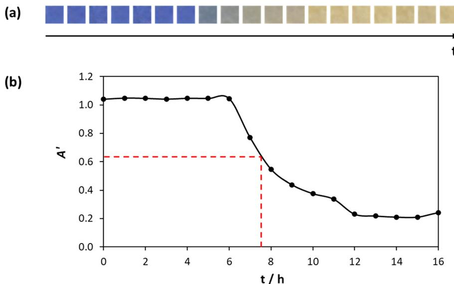
Fig. 4 (a) Photographs of the XB/silicone indicator in a typical CO<sub>2</sub>  $\mu$ R-TVC experiment using a 10<sup>4</sup> CFU mL<sup>-1</sup> inoculum of *E. coli* and (b) plot of the results of DCA analysis of the images in (a) in the form of  $A'$  vs.  $t$ . The red, broken horizontal and vertical lines highlight the time point (TT) when the sensor is half-way through its colour change.
