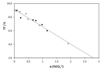
Fig. 5 Plot of TT vs. CO<sub>2</sub> sensor sensitivity (α) using data taken from Table 1. The open and closed circles refer to water and solvent based CO<sub>2</sub> sensors, respectively. The gradient and intercept of the line of best fit to all the data are  $-2.54 \pm 0.16$  and  $9.13 \pm 0.12$ , respectively.
