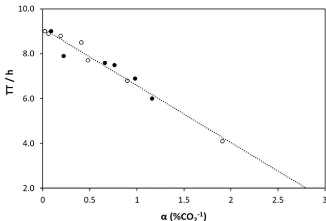
Fig. 5 Plot of TT vs. CO<sub>2</sub> sensor sensitivity ( $\alpha$ ) using data taken from Table 1. The open and closed circles refer to water and solvent based CO<sub>2</sub> sensors, respectively. The gradient and intercept of the line of best fit to all the data are  $-2.54 \pm 0.16$  and  $9.13 \pm 0.12$ , respectively.
