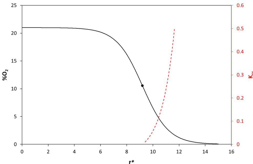
**Fig. 1** Plot of %O<sub>2</sub> vs. unitless time parameter  $t^*$ , calculated using eqn (3), assuming  $N_{\max}$  and  $N_0$  are  $10^8$  and  $10^4$  CFU mL<sup>-1</sup>, respectively. The broken red line is a plot of the variation in  $t_{\text{T}}^*$  for a series of O<sub>2</sub> sensors with different  $K_{\text{SV}}$  values, calculated using eqn (3) and (4). The black point marks the  $t^*$  value (9.2), =  $t_{1/2}^*$ , when  $N_0/N_{\max} = 0.5$  and %O<sub>2</sub> = 10.5%.
