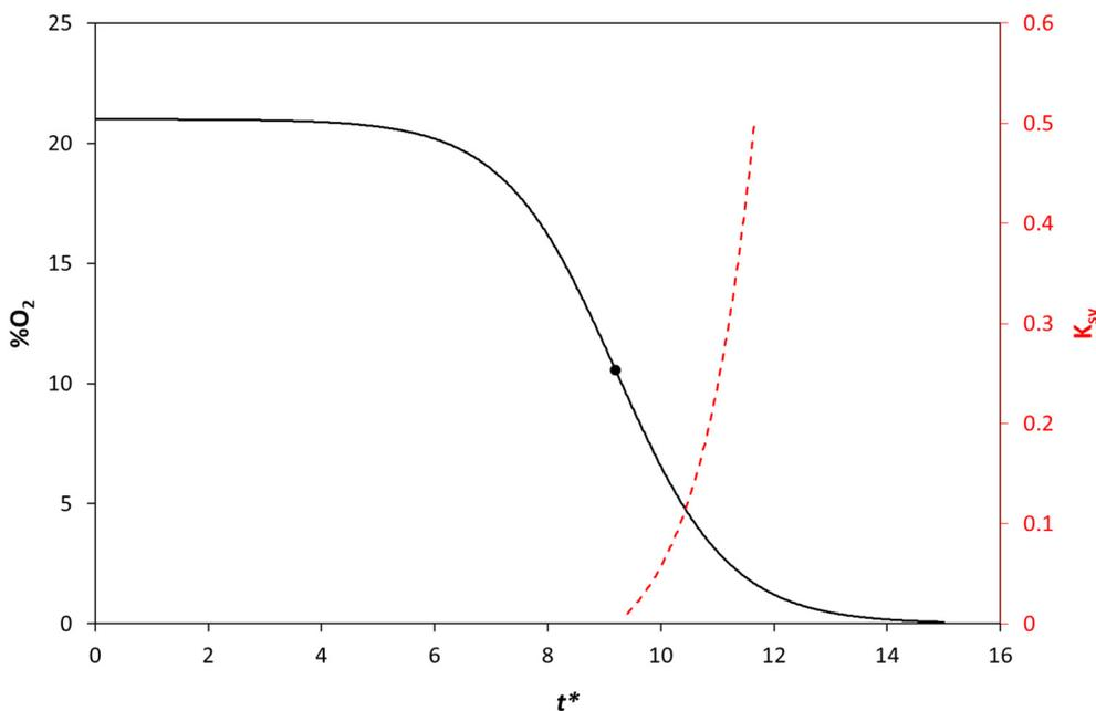
**Fig. 1** Plot of %O<sub>2</sub> vs. unitless time parameter  $t^*$ , calculated using eqn (3), assuming  $N_{\max}$  and  $N_o$  are  $10^8$  and  $10^4$  CFU mL<sup>-1</sup>, respectively. The broken red line is a plot of the variation in  $t_{TT}^*$  for a series of O<sub>2</sub> sensors with different  $K_{SV}$  values, calculated using eqn (3) and (4). The black point marks the  $t^*$  value (9.2), =  $t_{1/2}^*$ , when  $N_o/N_{\max} = 0.5$  and %O<sub>2</sub> = 10.5%.
