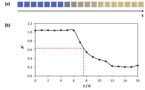
Fig. 4 (a) Photographs of the XB/silicone indicator in a typical CO<sub>2</sub>  $\mu$ R-TVC experiment using a 10<sup>4</sup> CFU mL<sup>-1</sup> inoculum of *E. coli* and (b) plot of the results of DCA analysis of the images in (a) in the form of A' vs. t. The red, broken horizontal and vertical lines highlight the time point (TT) when the sensor is half-way through its colour change.
