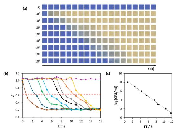
Fig. 6 (a) Photographic images of the XB/silicone indicator in a CO<sub>2</sub> µR-TVC study, in which the bacterial load of E. coli was varied over the range 108 to 101 CFU mL<sup>-1</sup>, (b) plots of A' vs. t for each different inoculum, calculated using DCA analysis of the images in (a) and eqn (8) (the red broken line highlights the mid colour-change point which was used to derive values for TT for each inoculum), (c) plot of the log(CFU mL<sup>-1</sup>) vs. TT data derived from (b).
