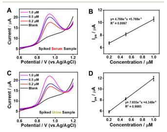
Fig. 7 DPV curves of NiMn<sub>2</sub>O<sub>4</sub>/CNT-GCE obtained for (A) spiked human serum and (C) spiked urine samples with increasing MTX concentrations in 0.1 M PBS (pH 7.0). (B) and (D) show the corresponding linear plots between  $I_{pa}$  and MTX concentrations for the serum and urine samples, respectively.
