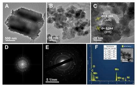
Fig. 3 (A and B) TEM image of NiMn<sub>2</sub>O<sub>4</sub>/CNT (C) HR-TEM of NiMn<sub>2</sub>O<sub>4</sub>/CNT nanocomposite. (D) FFT pattern of NiMn<sub>2</sub>O<sub>4</sub>/CNT, (E) SAED pattern and (F) EDS analysis of the NiMn<sub>2</sub>O<sub>4</sub>/CNT nanocomposite (inset: corresponding TEM image of the analyzed area and the EDS elemental composition table).
