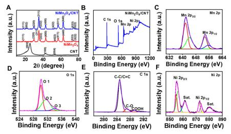
Fig. 1 (A) XRD patterns of CNT, NiMn<sub>2</sub>O<sub>4</sub>, and NiMn<sub>2</sub>O<sub>4</sub>/CNT. (B) XPS survey spectrum of NiMn<sub>2</sub>O<sub>4</sub>/CNT. (C–F) High-resolution XPS spectra of NiMn<sub>2</sub>O<sub>4</sub>/CNT: (C) Mn 2p, (D) O 1s, (E) C 1s, and (F) Ni 2p.
