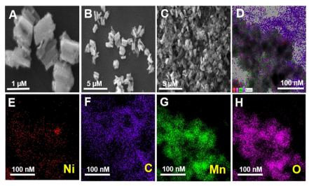
Fig. 2 SEM images of (A and B) NiMn<sub>2</sub>O<sub>4</sub> at different magnification (C) NiMn<sub>2</sub>O<sub>4</sub>/CNT. (D-H) Elemental mapping analysis of the NiMn<sub>2</sub>O<sub>4</sub>/CNT nanocomposite showing elements Ni, C, Mn, and O.
