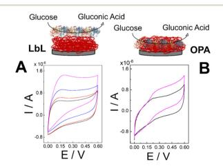
Fig. 3 (A) CVs performed for (PQQ-GDH/PDA)<sub>LbL</sub>/G in 10 mM HEPES buffer pH 7.2 + 100 mM KCl at 2 mV s<sup>-1</sup> containing 0 mM (black curve), 1 mM (red curve), 5 mM (blue curve) and 10 mM (magenta curve) D-glucose (inset: scheme of (PQQ-GDH/PDA)<sub>LbL</sub>/G); (B) CVs performed for (PQQ-GDH/PDA)<sub>OPA</sub>/G in 10 mM HEPES buffer pH 7.2 + 100 mM KCl at 2 mV s<sup>-1</sup> containing 0 mM (black curve) and 10 mM (magenta curve) D-glucose (inset: scheme of (PQQ-GDH/PDA)OPA/G).
