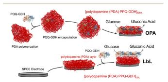
Fig. 1 Scheme of the deposition protocol for (PQQ-GDH/PDA)<sub>OPA</sub>/G and (PQQ-GDH/PDA)LbL/G electrodes.
