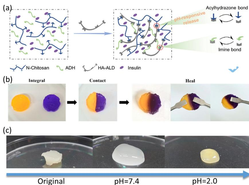
**Fig. 8** (a) Synthesis and pH response process of insulin-loaded hydrogels. Reproduced from ref. 148 with permission. (b) Self-healing photos of OHbG/QCMCS hydrogels. (c) Image of OHbG/QCMCS hydrogel in the drug release test. Reproduced with permission from ref. 151. Copyright 2025, MDPI.
