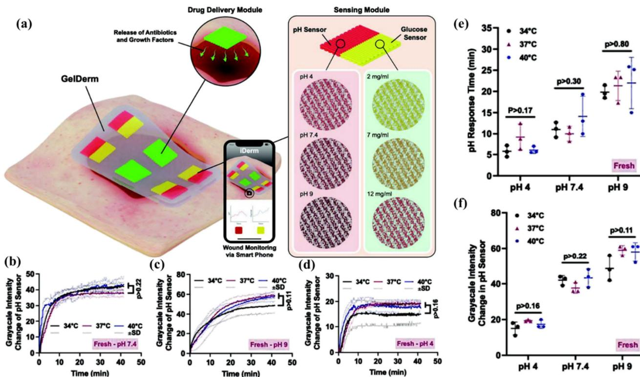
Fig. 10 (a) Schematic of GelDerm showing its integrated arrays of drug-releasing and sensing modules. (b–d) Variation of the gray intensity of the pH sensor with time at temperatures from 34 to 37 °C in a buffer solution environment with a pH range of 4 to 9. The changes of gray intensity (e) and response time (f) at different pH values from 34 °C to 37 °C were studied. Reproduced with permission from ref. 163. Copyright 2023, Wiley-VCH GmbH.
