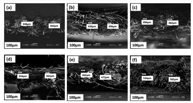
Fig. 5 Cross sectional SEM images of the: (a) cotton textile, (b) cotton textile coated with 5% GNP/NiFe<sub>2</sub>O<sub>4</sub>, (c) cotton textile coated with 10% GNP-NiFe<sub>2</sub>O<sub>4</sub>, (d) cotton/polyester mix textile, (e) cotton/polyester mix textile coated with 5% GNP-NiFe<sub>2</sub>O<sub>4</sub>, and (f) cotton/polyester mix textile coated with 10% GNP-NiFe2O4.
