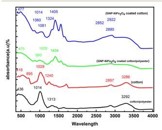
Fig. 2 FTIR spectra of non-coated and coated textiles with the GNP-NiFe<sub>2</sub>O<sub>4</sub> composite.
