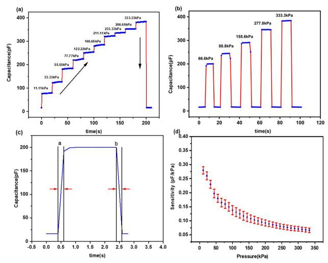
Fig. 7 The capacitive response of the sensor under: (a) step loading and (b) loading and unloading, (c) response and recovery time, and (d) sensitivity of five sensors under applied pressure, representing the average and spread.
