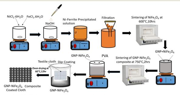
Fig. 1 Synthesis of the GNP-NiFe<sub>2</sub>O<sub>4</sub> composite and formulation process of paste for coating on cloth.
