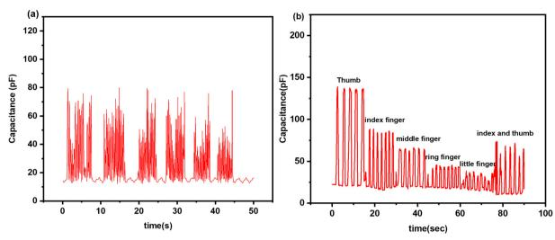
Fig. 8 Testing of the sensor by tapping with (a) the index finger and (b) all fingers of the right hand.
