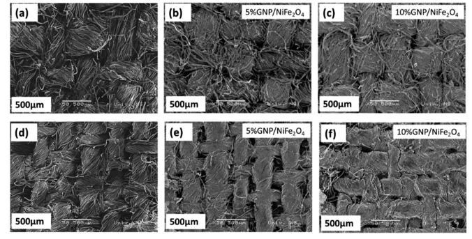
Fig. 4 SEM images of: (a) cotton textile, (b) cotton textile coated with 5% GNP-NiFe<sub>2</sub>O<sub>4</sub>, (c) cotton textile coated with 10% GNP-NiFe<sub>2</sub>O<sub>4</sub>, (d) cotton-polyester textile, (e) cotton-polyester textile coated with 5% GNP-NiFe<sub>2</sub>O<sub>4</sub>, (f) cotton/polyester textile coated with 10% GNP-NiFe<sub>2</sub>O<sub>4</sub>.
