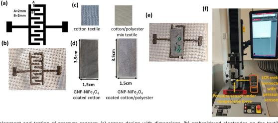
Fig. 3 Development and testing of pressure sensors: (a) sensor design with dimensions, (b) embroidered electrodes on the textile with a silver thread, (c) cotton and cotton/polyester mix textile, (d) cotton and cotton/polyester mix textile coated with GNP-NiFe<sub>2</sub>O<sub>4</sub>, (e) final sensor, coated textile attached with embroidered electrodes and sealed with PET, and (f) experimental setup to record the capacitance change due to a variation in applied pressure.
