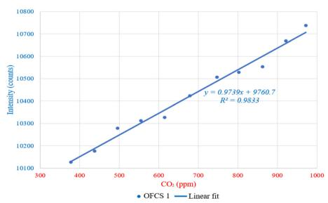
Fig. 9 Linear fitting of reflection intensities of OFCS 1 to different CO<sub>2</sub> concentrations at a wavelength of 600 nm.
