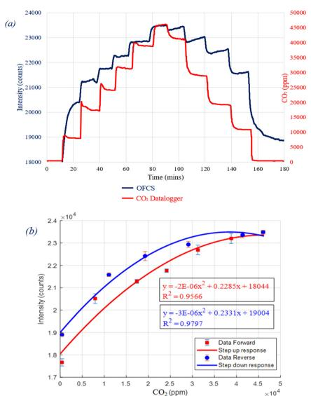
Fig. 7 Step-up and down response of the OFCS at a wavelength of 600 nm for different CO<sub>2</sub> concentrations; a) response with time; b) polynomial fitting of reflection intensities of the OFCS responses with increasing and decreasing CO<sub>2</sub> concentrations.
