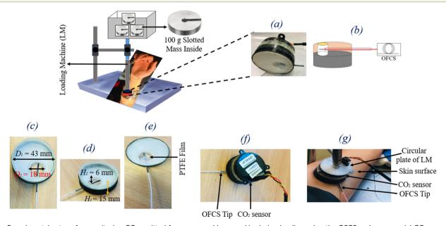
Fig. 3 Experimental set-up for monitoring CO<sub>2</sub> emitted from wrapped human skin during loading using the OFCS and commercial CO<sub>2</sub> sensor: (a) magnified image, (b) schematic diagram, (c) top view, (d) side view, and (e) bottom view of the PLA holder and top view of this holder on (f) a wooden surface without a loading arm and (g) a skin surface with a loading arm.
