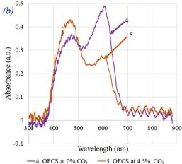
Fig. 6 (a) Reflection spectra of the OFCS; black line 1, reference signal from the reflection spectrum of the bare fibre; red line 2, intensity of the OFCS at minimum concentration; green line 3, intensity of the OFCS at maximum concentration. (b) Absorption spectra of the OFCS; purple line 4, absorbance of the OFCS at minimum concentration; orange line 5, absorbance of the OFCS at maximum concentration.
