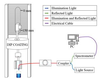
Fig. 1 Experimental set-up for the coating process onto an optical fibre tip
