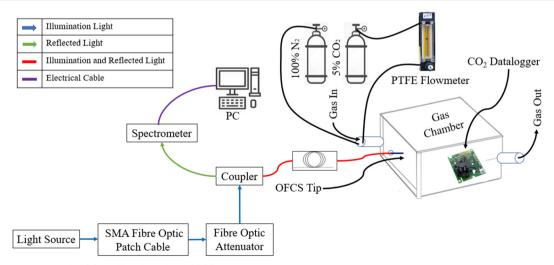
Fig. 2 Experimental set-up for CO<sub>2</sub> calibration of the OFCS.
