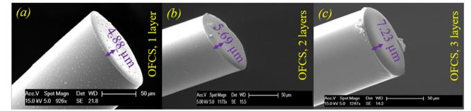
Fig. 4 SEM images of the OFCS tip with (a) 1 layer, (b) 2 layers and (c) 3 layers. Scale bar =  $50 \mu m$ .
