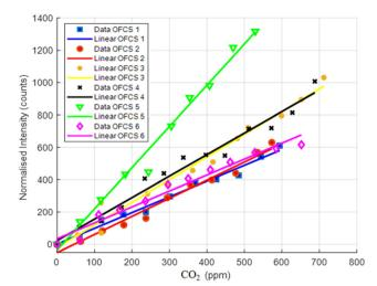
Fig. 10 Linear fitting of normalised intensities of 6 OFCSs (OFCS 1-6) to different CO<sub>2</sub> concentrations at a wavelength of 600 nm.
