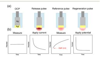
Fig. 1 Illustration of the principle (a) and potential and current
