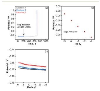
Fig. 4 Potentiometric traces for the deposition of the silver iodide layer, corresponding to a conversion of 30% of the silver layer (a). Response to changes in iodide activity (b) and reference values produced by the pulstrode protocol (c) of electrodes with 30%
