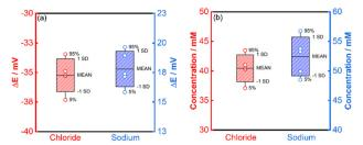
Fig. 7 Potentiometric quantification of urine ions using inkjet-printed electrodes (N=5) (a) potential differences between synthetic (calibrant) and biological urine and (b) concentration measured in biological urine.
