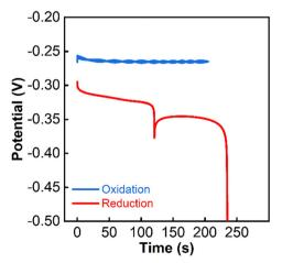
Fig. 5 Potentiometric traces under application of galvanostatic currents of 15.7 (blue) and –15.7  $\mu A$  (red) in 0.1 M NaI solution for one inkjet-printed electrode.
