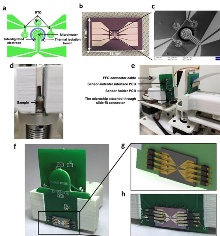
**Fig. 5** (a) Microchip design, (b) optical photograph of the fabricated microchip, (c) SEM image of the active area of the microchip, (d) sample loaded in the system, (e) subsystem with the PCBs, (f) microchip packaged into the sensor holder structure through slide-fit contacts, (g and h) rendered and actual image of the microchip connected to the slide-fit contacts. Reproduced from ref. 88 published under the terms and conditions of Creative Commons Attribution 4.0 International license.
