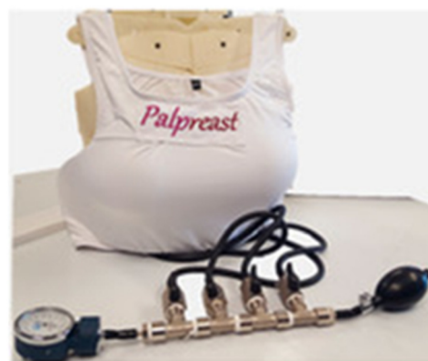
Fig. 6 Prototype design of the Palpreast device, including a smart wearable and inflator system. Reproduced from ref. 89 published under the terms and conditions of the Creative Commons Attribution (CC BY) license.
