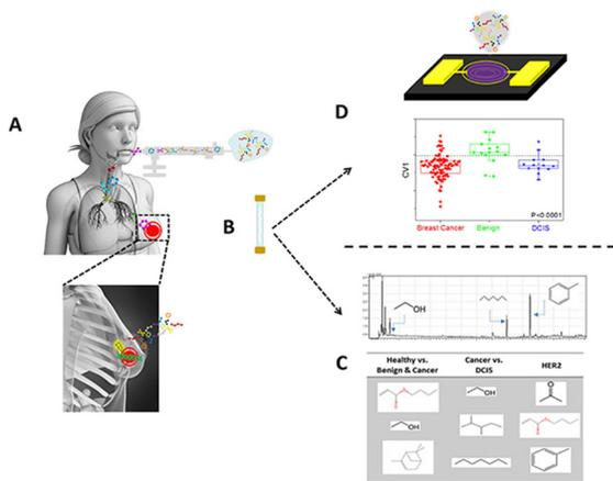
**Fig. 4** (A) Patient exhales into a collection bag. (B) Collection and concentration of breath on Tenax® (C) exposure of the Tenax® tube to GC-MS for detecting the presence of specific compounds. (D) Exposure to the AI nanoarray for volatolomic signature of BrC genetic mutations. Reproduced from ref. 77 published under the terms and conditions of the Creative Commons Attribution license.
