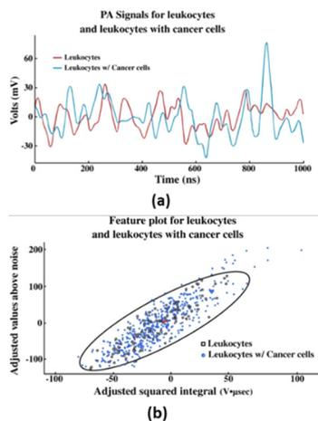
**Fig. 2** (a) PA waveforms obtained from the PAFC test from centrifuged blood. (b) Feature plot of each PA waveform from leukocytes and leukocytes with cancer cells. Reproduced from ref. 29. Published under the terms and conditions of the Creative Commons Attribution 4.0 Unported license.
