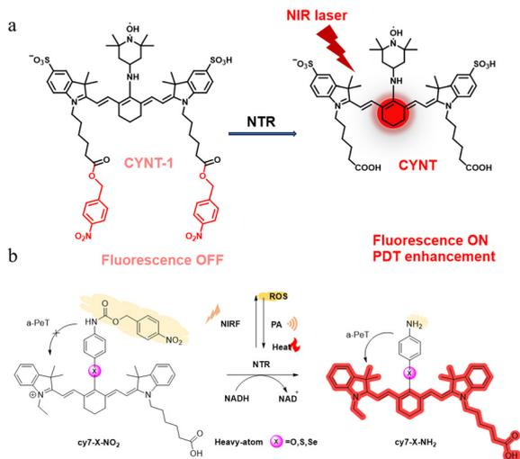
**Fig. 3** (a) The structure of CYNT-1 and its deduced enzyme-catalyzed mechanism activated with NTR. Reproduced with permission.<sup>38</sup> Copyright 2020 Royal Society of Chemistry. (b) Structures of Cy7-X-NH<sub>2</sub> and Cy7-X-NO<sub>2</sub> (X = O, S, Se), and response mechanism of Cy7-X-NO<sub>2</sub> toward NTR. Reproduced with permission.<sup>40</sup> Copyright 2024 Elsevier.
