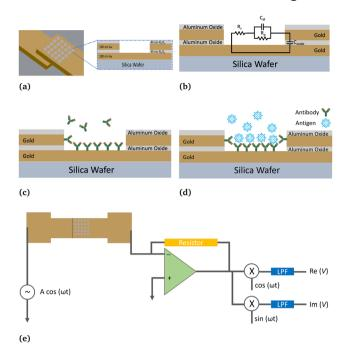
Fig. 1 (a) Cross-sectional view of a single nanowell. (b) Equivalent circuit model. (c) Cross-sectional view of single nanowell adsorbing antibodies. (d) Cross-sectional view of the nanowell adsorbing target proteins (e) Equivalent circuit of measurement platform using a lock-in amplifier.
