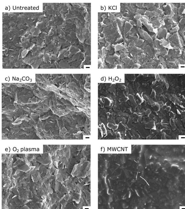
**Fig. 3** Top-view SEM images of screen-printed carbon electrodes a) without surface treatment and modified by b) KCl, c) Na<sub>2</sub>CO<sub>3</sub>, d) H<sub>2</sub>O<sub>2</sub>, or e) O<sub>2</sub> plasma exposure and f) by adding of 2 wt% multi-walled carbon nanotubes (MWCNT). The black scale bars correspond to 1 μm.
