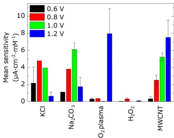
**Fig. 6** Mean glucose sensitivity of carbon working electrodes modified by either KCl, Na<sub>2</sub>CO<sub>3</sub>, O<sub>2</sub> plasma, H<sub>2</sub>O<sub>2</sub> or multi-walled carbon nanotubes with different applied working potentials 0.6 V (black), 0.8 V (red), 1.0 V (green) and 1.2 V (blue) vs. the Ag/AgCl reference electrode.
