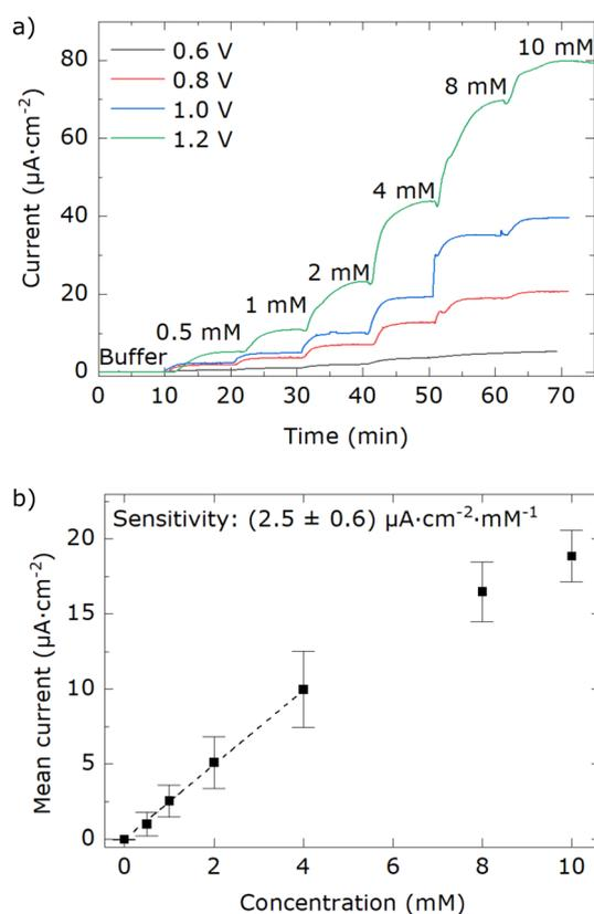
**Fig. 5** a) Dynamic response of carbon working electrodes with 2 wt% MWCNTs with immobilized glucose oxidase to different glucose concentrations (0.5–10 mM) at different applied potentials 0.6 V (black), 0.8 V (red), 1.0 V (blue) and 1.2 V (green) vs. the Ag/AgCl reference electrode. b) Mean calibration plot with  $n = 5$  sensors at an applied potential of 0.8 V vs. the Ag/AgCl reference electrode.
